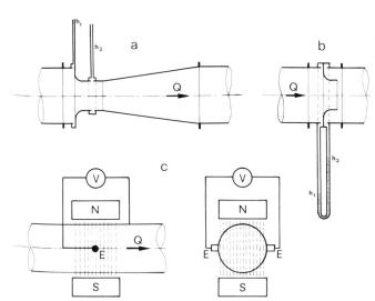
Reference number 2.202. Measurement of flow in pipes. (a) Venturi meter, (b) Flow nozzle, (c) Electromagnetic flowmeter; (N, S) Poles of the magnetic field, (E) Electrodes, (V) Voltmeter for measuring the induced voltage which is proportional to the average velocity of the fluid, (Q) Discharge.
