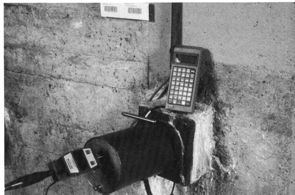
Reference number 2.120-1(2). Rod extensometer for concrete dams. Measuring head for measurements by hand (using a digital dial gauge) and with digital data registration and identification of the measuring points.
