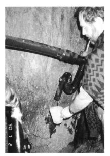
Reference number 2.200(3). Drainwater measurement by means of a calibrated container
