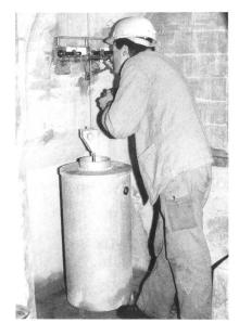
Reference number 2.100(3). Measuring of dam deflection at the bottom of a plumb line. The weight is enclosed in a tank filled with oil or water.
