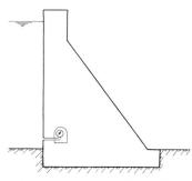
Reference number 1.000-4. Manometer to measure the hydrostatic pressure corresponding to the reservoir water level.
