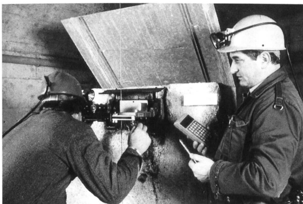
Reference number 2.100(5). Optical sighting of the plumb line position and digital data registration and identification of the measuring point.
