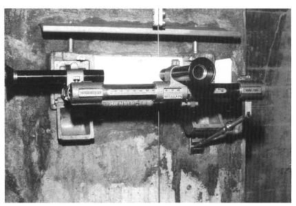
Reference number 2.100(4). Optical instrument to read the position of the plumb line wire with the help of a vernier scale.
