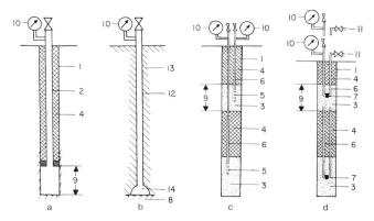
Reference number 2.301-1(1). Closed borehole measuring equipment for concrete dams. (a) Simple pipe, (b) Pipe with uplift bell, (c) Pipe with filters, (d) Tubes with rinsable measuring cells; 1 Borehole, 2 Pipe (diameter 2" to 2,5"), 3 Sand, 4 Grout, 5 Porous filter, 6 Flexible tube (internal diameter 8 to 12 mm), 7 Measuring cell, 8 Foundation rock, 9 Measuring section, 10 Manometer, 11 Flushing stop-cock, 12 Embedded pipe (diameter 2" to 2,5"), 13 Concrete, 14 Bell.
