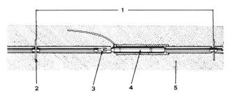
Reference number 2.120-2. Rod extensometer for embankment dams. 1 Measurement lenght, 2 Anchor plate, 3 Flexible joint, 4 Measuring element (extensometer unit), 5 Fill material [Hanna 1985].
