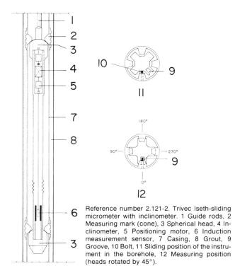
(The grouting between the tubing and the wall of the borehole must be carried out very carefully.)
