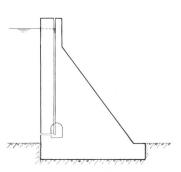
Reference number 1.000-5. Acoustic or light gauges to measure the reservoir water level.
