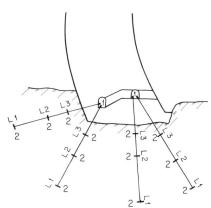
Reference number 2.120-1(4), above. Possible arrangement of extensometers in the foundation of an arch dam showing four borings equiped with three extensometers anchored at different depths.
