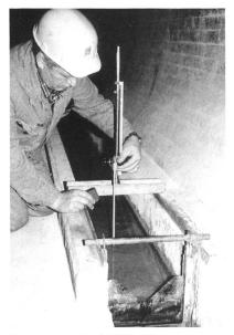
Reference number 2.201(1). Triangular weir in a seepage channel. To measure the discharge, the water level is determined by means of a measuring pointer.
