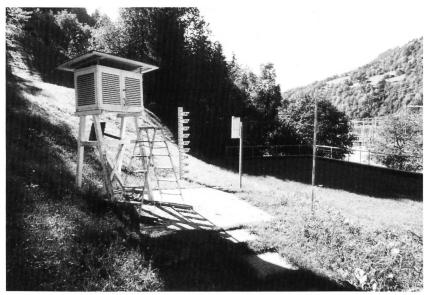
Reference number 1.200. Pluviometer (center of the photograph) integrated in a meteorological field station.
