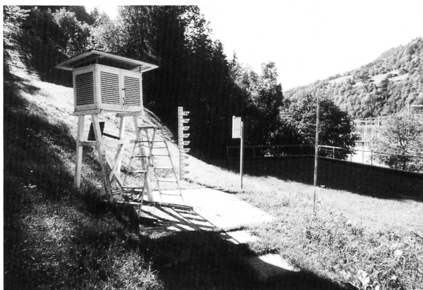
Reference number 1.200. Pluviometer (center of the photograph) integrated in a meteorological field station.
