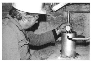
Reference number 2.120-1(1). Rod extensometer for concrete dams Measuring head with mechanical and electrical reading.
