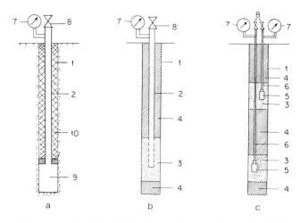
Reference number 2.301-2. Closed borehole measuring equipment for embankment dams. (a) Simple pipe, (b) Standpipe, (c) Casagrande-type piezometer; 1 Borehole, 2 Pipe (diameter 2" to 2,5"), 3 Sand, 4 Impervious fill, 5 Porous filter, 6 Flexible tube (internal diameter 8 to 12 mm), 7 Manometer, 8 Pressure relief and flushing valve, 9 Measuring section in the rock. 10 Grout.
