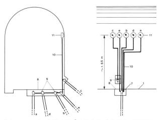
Reference number 2.301-1(3). Connections of pipes to manometers. Floor wall, 2 Grout, 3 Concrete, 4 Rock-concrete interface, 5 Tubed length of borehole, 6 Non-tubed borehole, 7 Ditch, 8 Metal cover, 9 T-piece (e.g. 2" to 2,5") acting as pipe closure and connection to pressure tube, 10 Flexible pressure tube, 11 Manometer.
