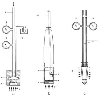
Reference number 2.302. Types of piezometric cells. (a) The pneumatic piezometer, (b) Vibrating wire piezometer, (c) Twin-tube hydraulic piezometer; 1 Gas supply tube, 2 Gas flow gauge, 3 Pressure gauge, 4 Membrane, 5 Porous filter, 6 Return tube, 7 Gas flow indicator, 8 Vibrating wire, 9 Electrical coil, 10 Signal cable, 11 Twin plastic tubes containing deaired water.
