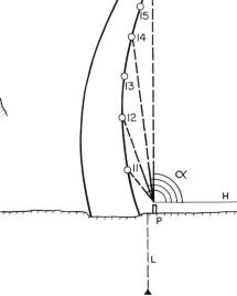
Reference number 2.101(2). Simple measurement of vertical angles used for determining the upstream/downstream deplacements of targets located on the downstream face of the dam. (P) Reference point, usually an observation pillar, (H) Horizon, (L) Inverted plumb line, 11 to 16 Control targets.
