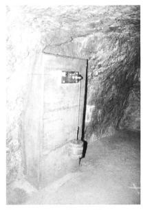
Reference number 2.110(3). Wire alignment. The weight spans the wire constantly at one end
