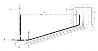
Reference number 3.102. Schematic of hose levelling device or overflow gage. 1 Measurement cell, 2 Water overflow tube, 3 Vent tube, 4 Drain tube, 5 Fixed graduated transparent tube, 6 Liquid level to be measured, 7 Supply of deaerated water to cause overflow in the cell
