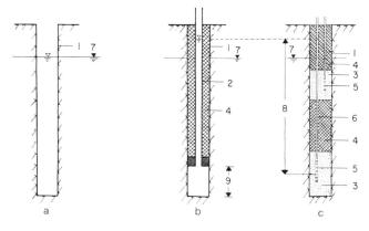
Reference number 2.300-1(1). Open borehole of standpipe measuring equipment for concrete dams. (a) Open borehole, (b) Standpipe, (c) Standpipe with filters; 1 Borehole, 2 Pipe (diameter 2" to 2,5"), 3 Sand, 4 Grout, 5 Porous filter, 6 Flexible tube (internal diameter 8 to 12 mm), 7 Phreatic water level, 8 Height of uplift, 9 Measuring section < 5 m.
