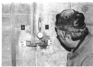
The reference points must be cleaned and greased periodically.
