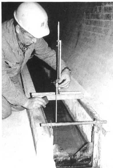
Reference number 2.201(1). Triangular weir in a seepage channel. To measure the discharge, the water level is determined by means of a measuring pointer.
