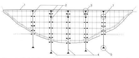
Reference number 2.1000(1), above. Typical example of a modern arrangement of plump lines. 1 Crest of dam, 2 Plumb line, 3 Point of suspension of plumb line, 4 Inverted plumb line, 5 Anchorage of inverted plumb line.
