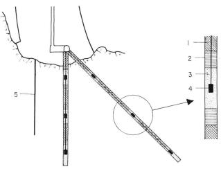
Reference number 2.301-1(6). Possible layout of uplift measurements of types (c) and (d) in the foundation of a dam. 1 Grout, 2 Clay pellets, 3 Quartz sand (grain size 1,5 to 2 mm), 4 Piezometer, 5 Grout curtain.
