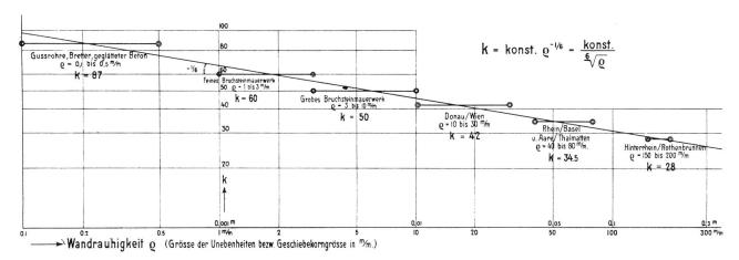
Figure 4. "Relationship between the k-values and the absolute wall roughness." Plate 17 of Strickler's treatise [1],  $\rho$  is the wall roughness that is the "size of the wall uneveness or of the bed load grains" ( $\rho = d$ ).
