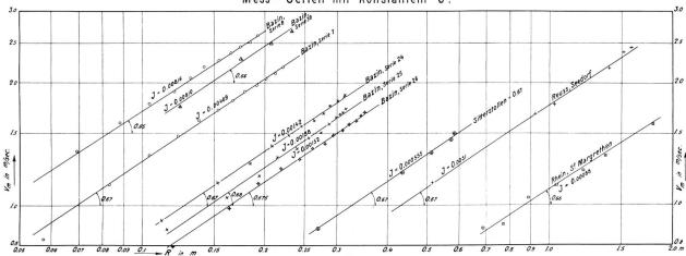
Figure 3. Above: "Determination of the exponent  $\mu$  in the formula  $v_m = k R^\mu J^\nu$ , measurement series with constant J." Below: "Determination of the exponent  $\nu$  in the formula  $v_m = k R^\mu J^\nu$ ; measurement series with constant R." Plates 4 and 5 of Strickler's treatise [1] (corresponding notation in the present note:  $v_m = v$ , J = S,  $\mu = a$ ,  $\nu = b$ ).
