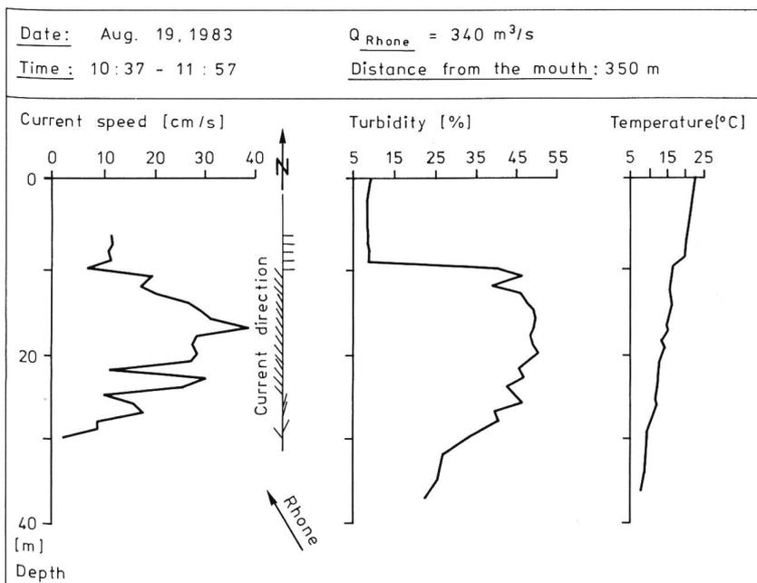
In order to study these phenomena in Lake Geneva an ultrasonic current meter was first of all applied to detect and measure the interflow of the Rhone river occurring close to the thermocline (at depths of 10 to 30m) during the period of lake water stratification. The results of this study mainly showed that currents caused by the momentum of the inflowing river water were clearly discernible up to a distance of about 1 km from the river mouth (figure 12).
