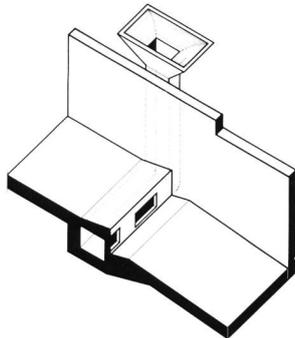
Figure 6. Aerator (ramp), supply system and air duct.
