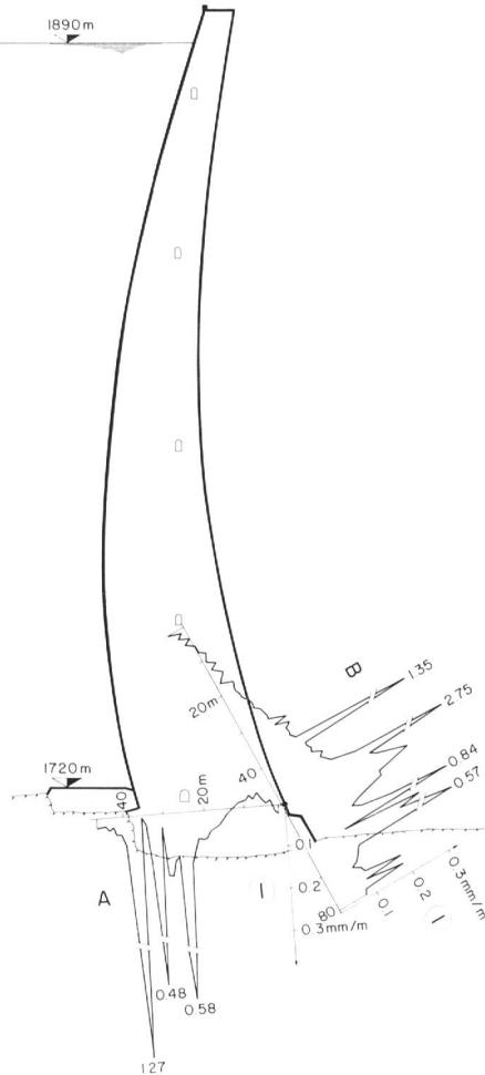
Figure 5. Kölnbrein, arch dam, block 18. Sliding micrometer, measuring results.
