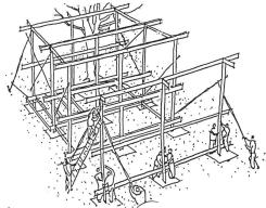
Hird frame plumbed and Braced to other twolast frame raised - ofter bracing, next comes the roof...
