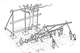
first frame plumbed upright - strutted to ground and any convenient tree - second frame raised -
