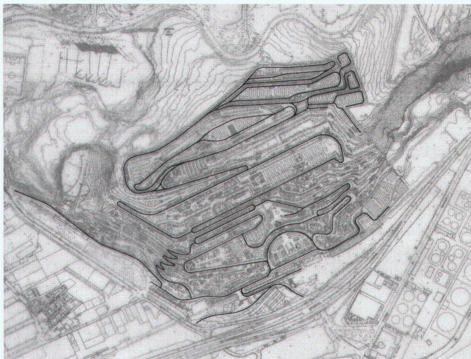
Analyseplan Terrassierung/Stützmauern ▷ Plan analytique terrasse- ment/soutènements ▷ Analytical plan of the terracing/supporting walls
