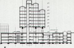
Construction. (High-rise office building, Cologne – 4-block building): The basic planning conception behind this office building and the necessity of having a generously dimensioned ground floor called for reinforced concrete construction. Reinforced concrete prefab parts are to be employed to the extent they can be meaningfully and economically integrated in the basic conception.
