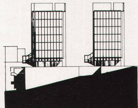
The experimental housing complex in Genoa consists of a solid primary structure of pre-stressed concrete and light, separately mounted wall elements as the secondary structure. The complex consists of 5 six-storey houses with common basement level
