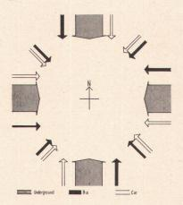
Directional capacity of transport modes Capacity shown by width of arrows available for immediate area SOURCE: Timetables, traffic survey
