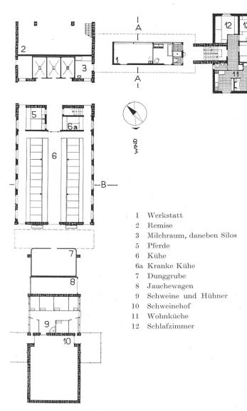
$Erdgescho\beta \ 1:400 \ | \ Rez\text{-}de\text{-}chauss\'{e}e \ | \ Ground\text{-}floor$
