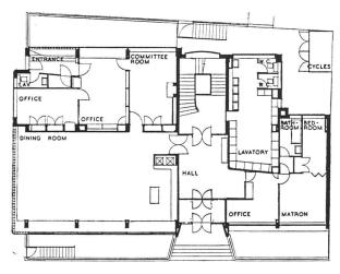
$Erdgescho\beta \ 1{:}\,300 \ | \ Rez\text{-}de\text{-}chauss\'{e}e \ | \ Groundfloor$
