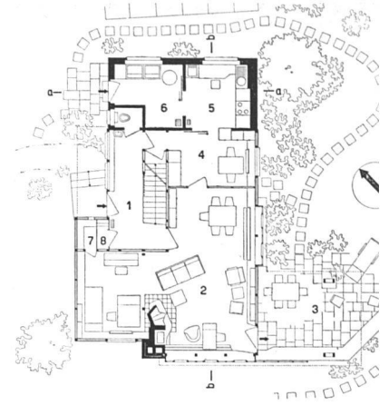
Erdgeschoß 1:300 | Rez-de-chaussée / Ground floor
