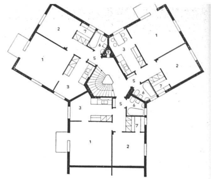
Normalgeschoß 1:400 | Plan d'étage type / Typical floor plan with three apartments
