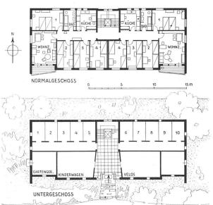
Grundrisse Blöcke A, B, C, D 1:400 | Plans des blocs A, B, C, D | Plans of blocks A, B, C, D
