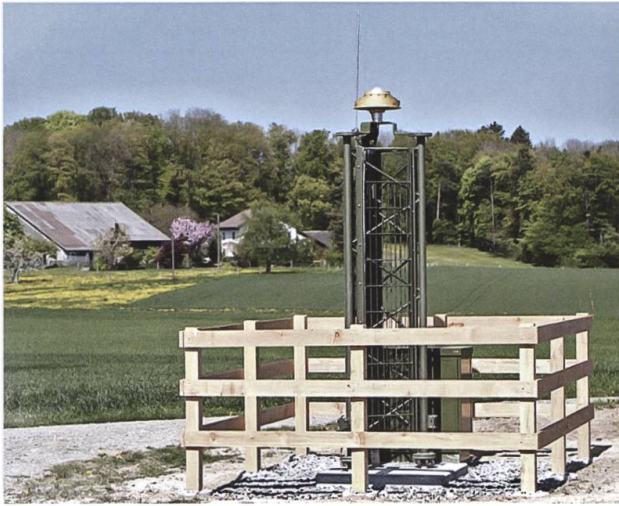
Fig. 3: Exemplary photograph of Nagra's permanent GNSS station Trüllikon (left) and exemplary time series from the north/east/up coordinates of Nagra's permanent GNSS station Seltisberg (right).
