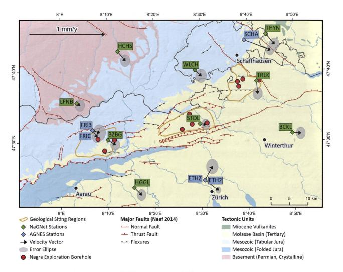
Fig. 4: Distribution of NaGNet and AGNES permanent GNSS stations in Northern Switzerland. Horizonal displacement rates (mm/y) with respect to the Swiss reference station Zimmerwald (ZIMM) are shown. Ellipses indicate uncertainties.
