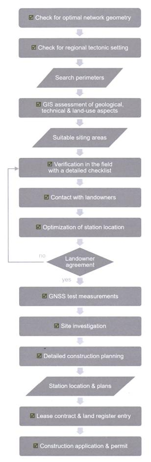
Fig. 1: Siting workflow for Nagra's permanent GNSS stations tracking geodynamic deformations in Northern Switzerland.
