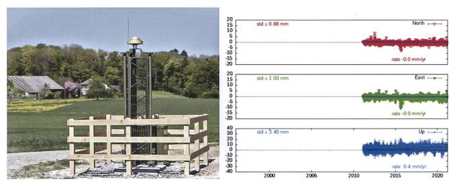
Fig. 3: Exemplary photograph of Nagra's permanent GNSS station Trüllikon (left) and exemplary time series from the north/east/up coordinates of Nagra's permanent GNSS station Seltisberg (right).
