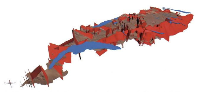
Fig. 1: Representation of the «Top Dogger» surface (brown) and fault zones (red) from the GeoMol19 model. View is from the SSW to NNE with a 3x vertical exaggeration. The model terminates along the southern edge of the Jura Mountains to the north, the Alps to the south, Lake Constance to the NE and Lake Geneva & France to the SW.
