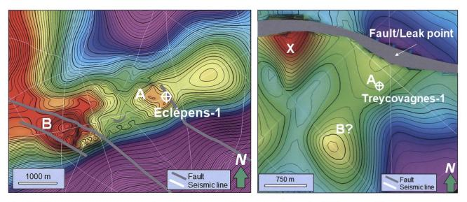
Fig. 12: 3D top reservoir structure of the target interval for storing CO2 at the Eclépens and Treycovagnes sites.
