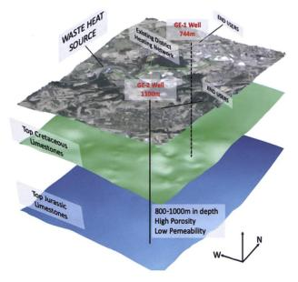
Fig. 8: Illustration of the Geneva project aiming to assess the heat storage potential for the devel-opment of an HT-ATES system connected to a waste-to-energy plant operated by Services Industriels de Genève (SIG).
