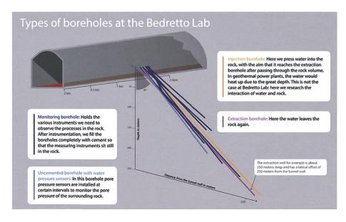
Fig. 7: Arrangement of boreholes and sensors for the Bedretto reservoir project.
