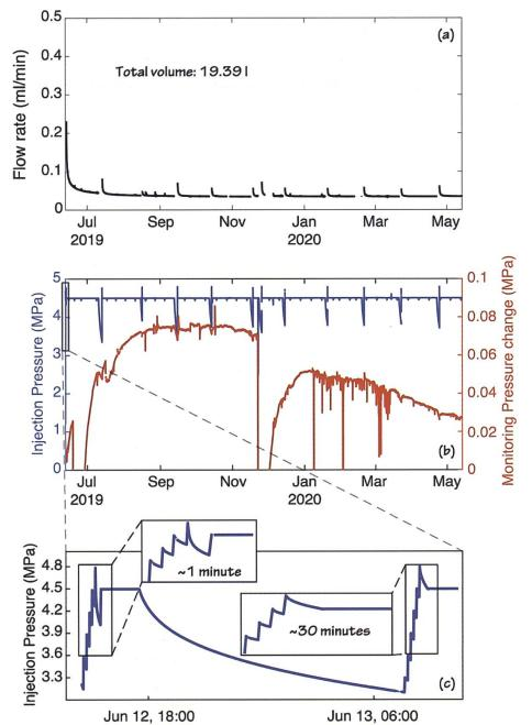
Fig. 13: (a) Flow rate recorded during the one year-long injection of CO2 saturated fluid. (b) Pressure at injection interval (blue line) and pressure changes recorded at the monitoring interval (red line). See Figure 1b for relative distances. (c) Zoom on injection pressure in the first days of injection.
