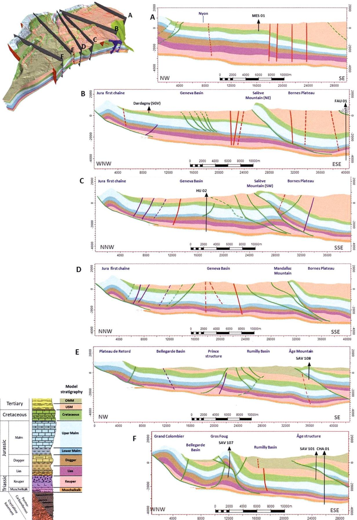
Fig. 6: Series of key regional cross-sections extracted from the 3D structural model of the study area. The main tectonic features discussed in the text are highlighted. The location of the profile is indicated in the inset figure at the top left. The stratigraphic layers indicated in the cross section correspond to the seismic horizons mapped for this work.
