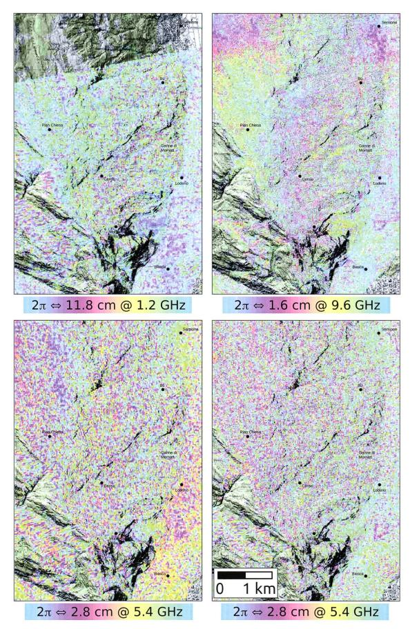
Fig. 3 left to right, top to bottom: DlnSAR from ALOS-2 PALSAR-2 between 2017.09.02 and 2017.10.28 (56 days, mean coherence 0.20), TerraSAR-X between 2017.09.23 and 2017.10.04 (11 days, mean coherence 0.15), Sentinel-1 between 2017.09.26 and 2017.10.08 (12 days, mean coherence 0.15) and Radarsat-2 between 2017.09.18 and 2017.10.12 (24 days, mean coherence 0.10). The legend indicates the apparent displacement corresponding to a phase cycle.
