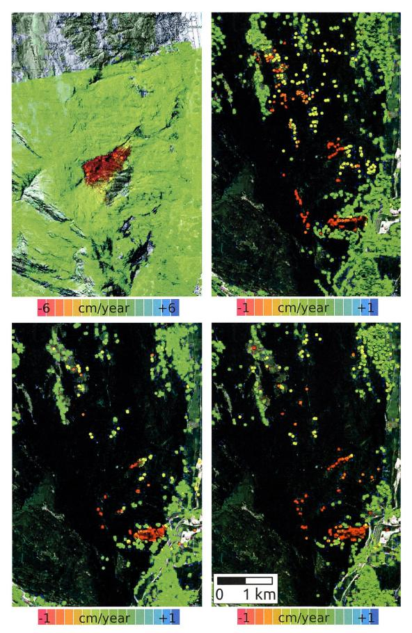
Fig. 5, left to right, top to bottom: MTI LOS displacement mapsfrom ALOS-2 PALSAR-2 between 2014 and 2018 and PSI LOS displacement maps from ALOS-2 PALSAR-2 between 2014 and 2018, TerraSAR-X between 2014 and 2017, SENTINEL-1 between 2015 and 2018 and Radarsat-2 between 2011 and 2017. The colour scale is saturated at 6 cm/year for ALOS-2 PALSAR-2 and at 1 cm/year for the three other sensors.
