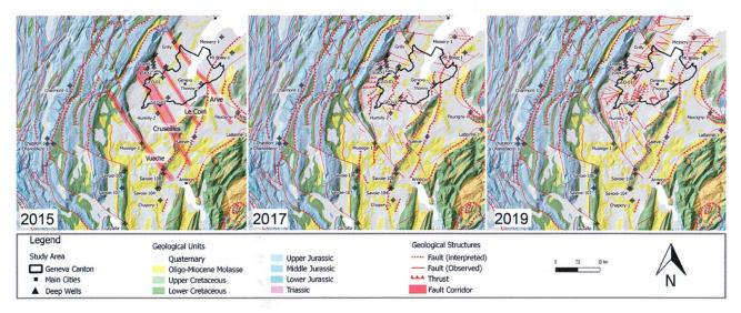
Fig. 6: Comparison of fault distribution in the Geneva Basin area based on the different and evolving views over the last 8 years (2013, 2017 and 2019). A higher complexity than previously thought seems to characterize the subsurface which will have important implications for effectively exploring and developing geothermal resources.
