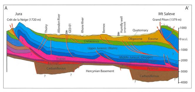
Fig. 3: Geological section crossing the Geneva Basin from SE to NW summarizing the key stratigraphic and structural elements present in the basin. This section has been drawn based on several 2D seismic lines and borehole data. See Figure 1 for the location of the A-A' trace.
