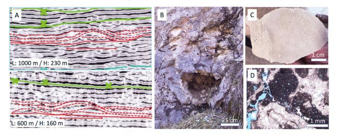
Fig. 5: Example of Kimmerdigian (Malm, Upper Jurassic) reef-complex reservoirs as they appear in A) 2D seismic in the subsurface of the Canton of Geneva (L and H indicates length and height, respectively), B) in outcrop (Prapont, Ain, France), C) hand-sample where specimens of ramose corals (Calamophyl- liopsis flabellum Michel) are well visible and D) thin section displaying carbonate reservoir with intrapar intraparticle porosity.
