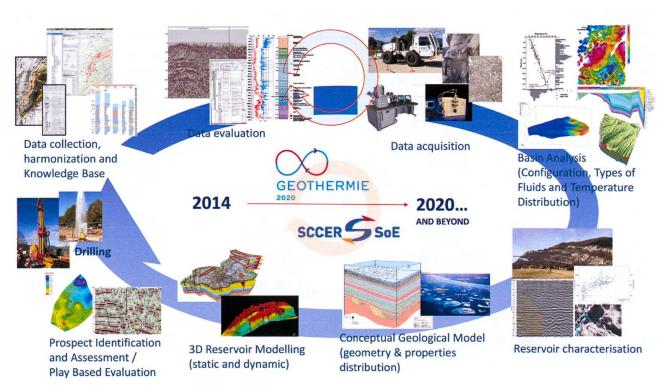
Fig. 2: Workflow and activities used in the geoenergy exploration phase aimed at the evaluation of geothermal resource potential. This workflow has been adopted to respond to the GEothermie 2020 program and the objectives of the large national swiss program SCCER SoE (Swiss Competence Center of Energy Research - Supply of Electricity) where fundamental research has been coupled to pilot and demonstration projects.
