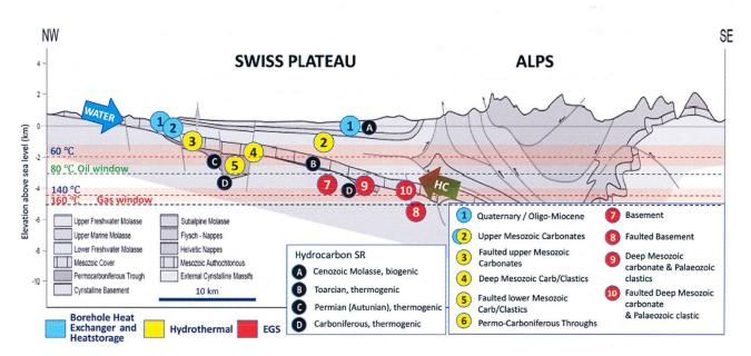
Fig. 4: Summary of geothermal and hydrocarbon plays on an ideal section across the Swiss Plateau. The circles with numbers indicate the different geothermal plays and the type of geothermal energy utilization (borehole heat exchange, heat-storage, hydrothermal and enhanced/engineered geothermal systems). The arrows indicate the main direction of water circulation in the subsurface which is primarily opposite to the up-dip migration of hydrocarbons.
