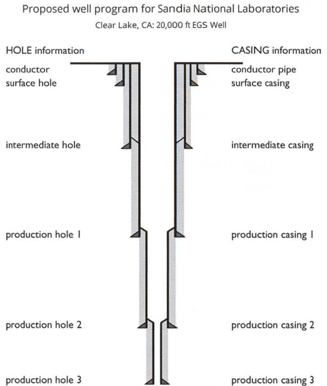
Fig. 13: Application of the DAT for Deep Well Borings - «Synthetic» Well from Sandia National Laboratories (after Polsky et al., 2008).
