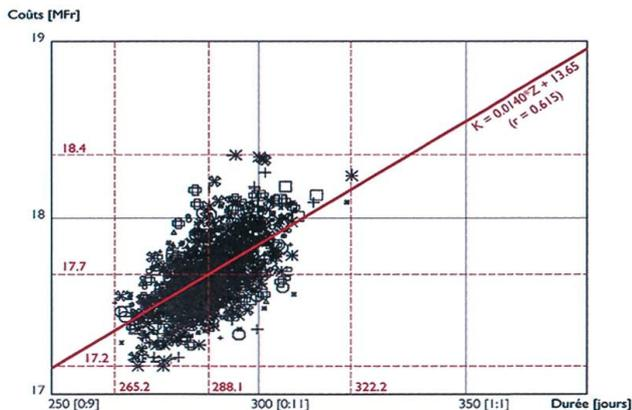
Fig. 2c: LBT Pilot Tunnel Frutigen- Mitholz – Resulting Cost - Time Scattergrams, Based on information from the contractor's bid.
