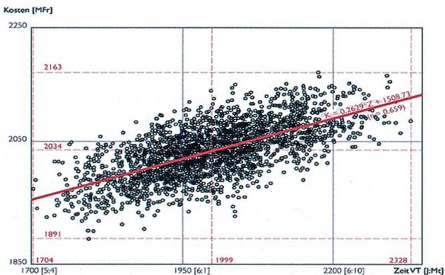
Fig. 4b: LBT 1997 Study of Cost and Time - Resulting Cost - Time Scattergrams, Variable mean unit costs and advance rates.
