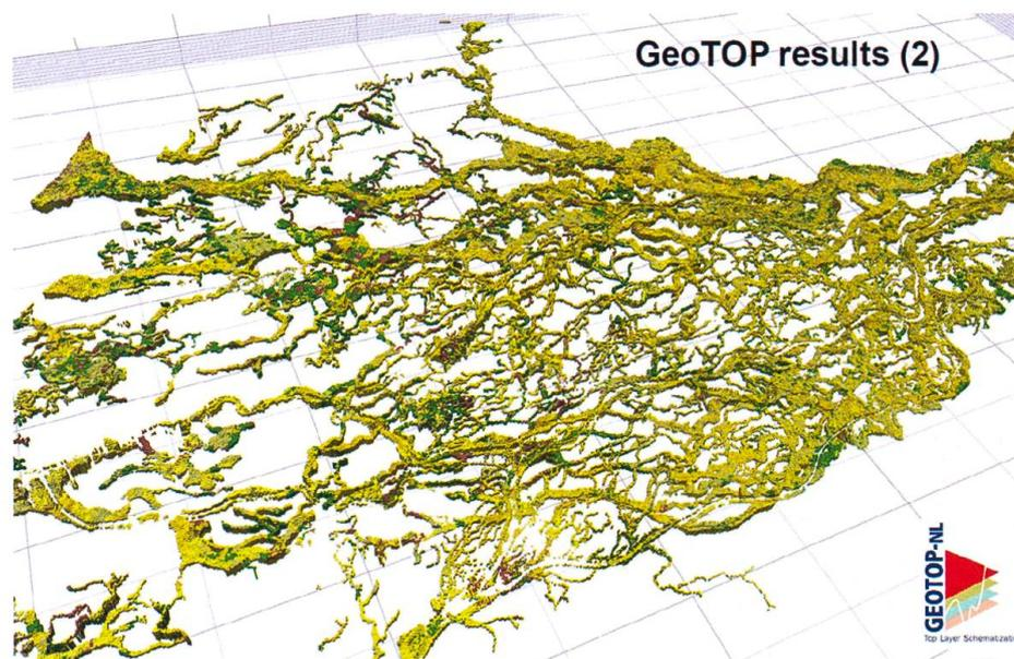
Fig. 3: The 3D voxel model GeoTOP (100 x 100 x 0.5 m) to a depth of 50 m.
