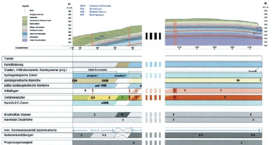
Fig. 5: KarstALEA profile of the Ligerz safety gallery with expected characteristics related to the karst aquifer and to the conduits (probability of occurrences, morphology of the conduits, hydrological regime, etc.).
