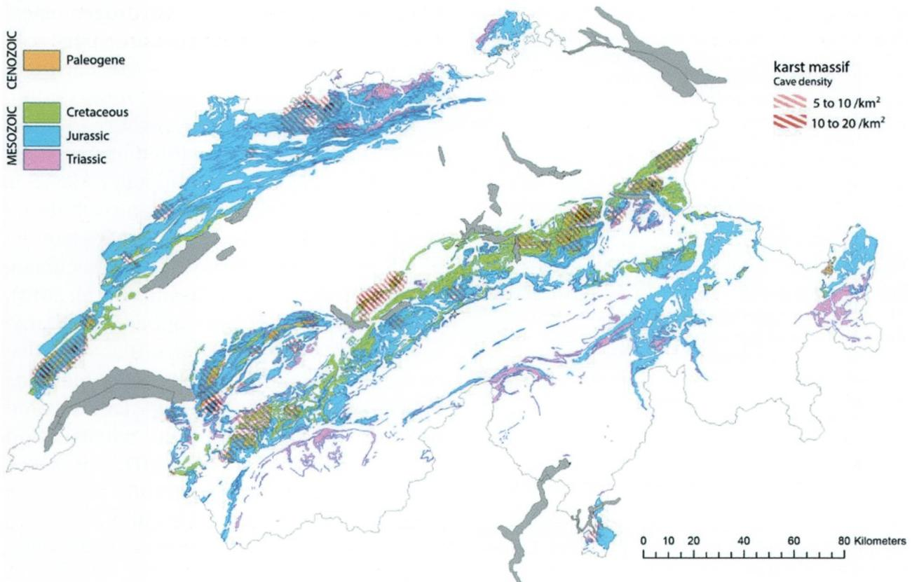
Fig. 1: Distribution of carbonate outcrops over the Swiss territory which may be potentially karstified. Red hatches locate high density cave areas [from 10 to 20 known entrances per km<sup>2</sup> for the most investigated sites]. Geological data comes from Swisstopo.
