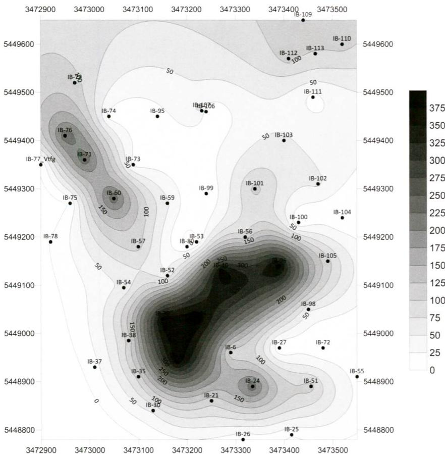
Fig. 10: Initial average production rates [bbl] of the Weiher field. Higher production rates can be correlated with larger reservoir thickness of a NE-SW trending channel fill and a NW-SE oriented fault defined by 3D seismic [production data compiled from Wirth 1950].
