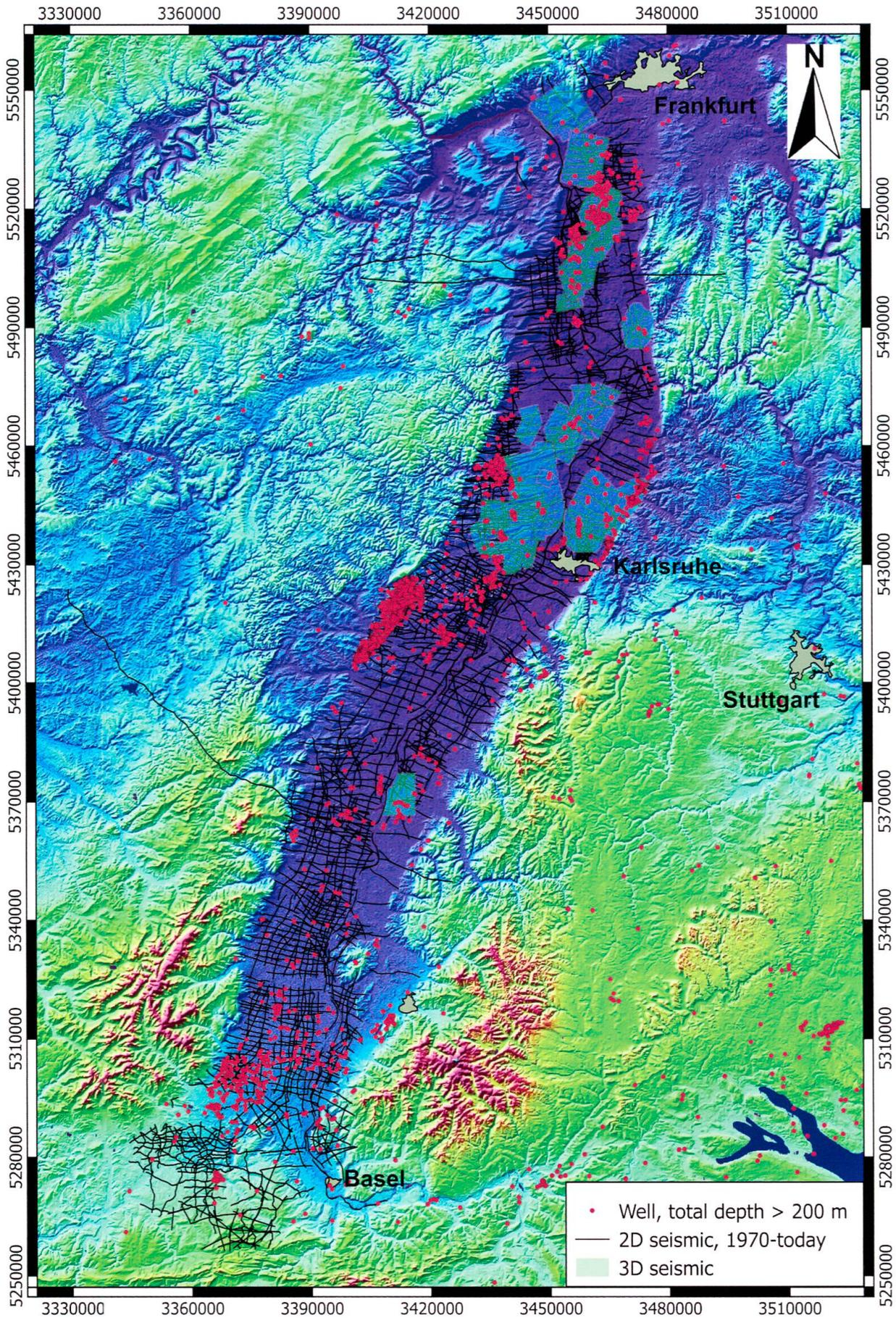
Fig. 1: Digital elevation model (DEM) of the Upper Rhine Graben (URG) and its graben shoulders including 2D and 3D seismic coverage and all wells with a total depth of  $\rightarrow$  200 m. DEM prepared by Geodetic Institute, Karlsruhe Institute of Technology, with SRTM data.
