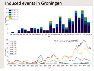
build-up in the reservoir rock. It is believed that accommodation of (a fraction of) this compaction strain by seismogenic fault slip is the source of the observed seismicity.
