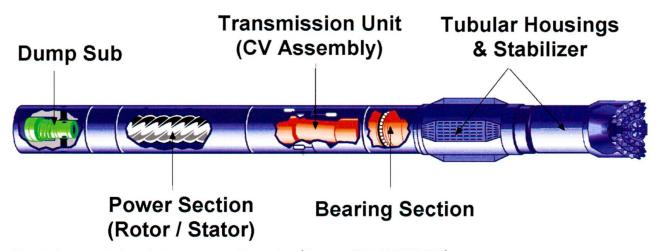
Fig. 2: A general downhole motor configuration (Source: HALLIBURTON).
