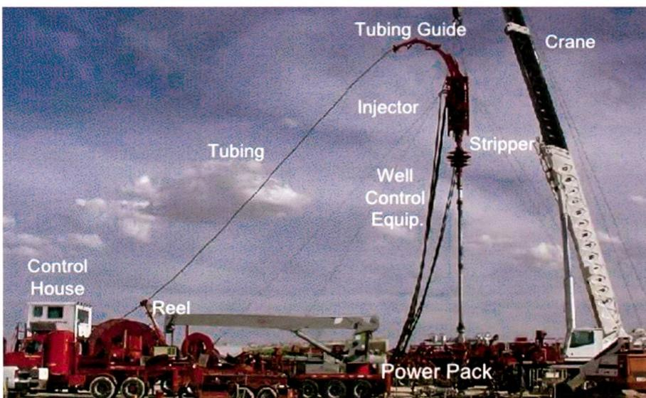
Fig. 4: Main components of CT unit [Source: HAL-LIBURTON].
