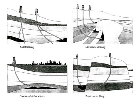
Fig. 1: Applications of directional drilling (Source: Weatherford).
