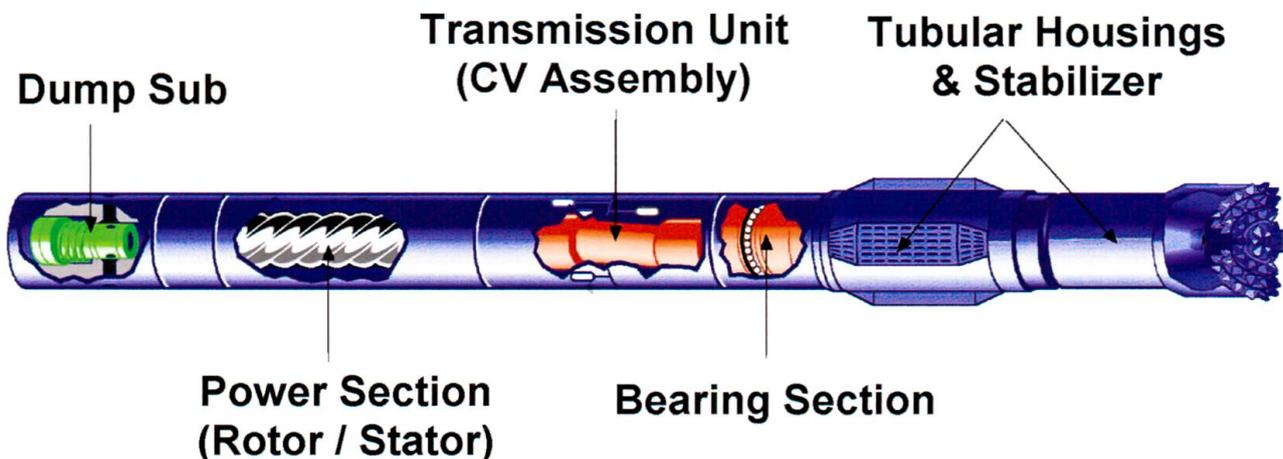
Fig. 2: A general downhole motor configuration (Source: HALLIBURTON).
