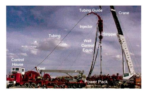
Fig. 4: Main components of CT unit (Source: HAL-LIBURTON).
