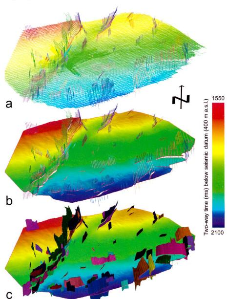
Fig. 1: Demonstration of the main steps in surface modelling in the time domain: a] Horizon interpretation (seed lines) of Base Mesozoic and fault sticks of the Mesozoic. bl unsmoothed horizon surface of Base Mesozoic and fault sticks of the Mesozoic and c] unsmoothed horizon surface of Base Mesozoic and water-tight fault surfaces of the Mesozoic. The orientation of the perspective 3D view is South to North and the vertical exaggeration of the time domain is three times.
