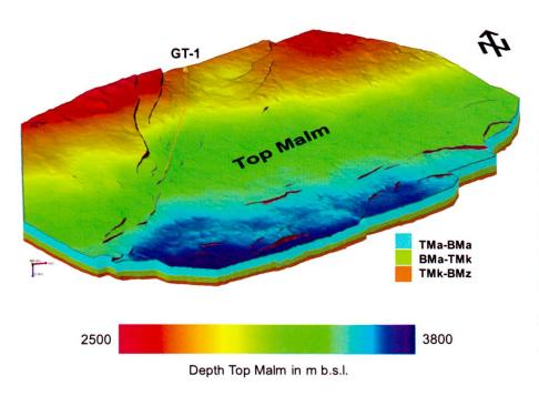
Fig. 3: Perspective view from South (no vertical exaggeration) of the 3D volume model with the layering of the Mesozoic in the depth domain (m a. s. l.). TMa-BMa: Interval Top Malm to Base Malm. BMa-TMk: Interval Base Malm to Top Muschelkalk. TMk-BMz: Interval Top Muschelkalk to Base Mesozoic. The depth map of Top Malm (TMa) is draped onto the model in illumination representation.
