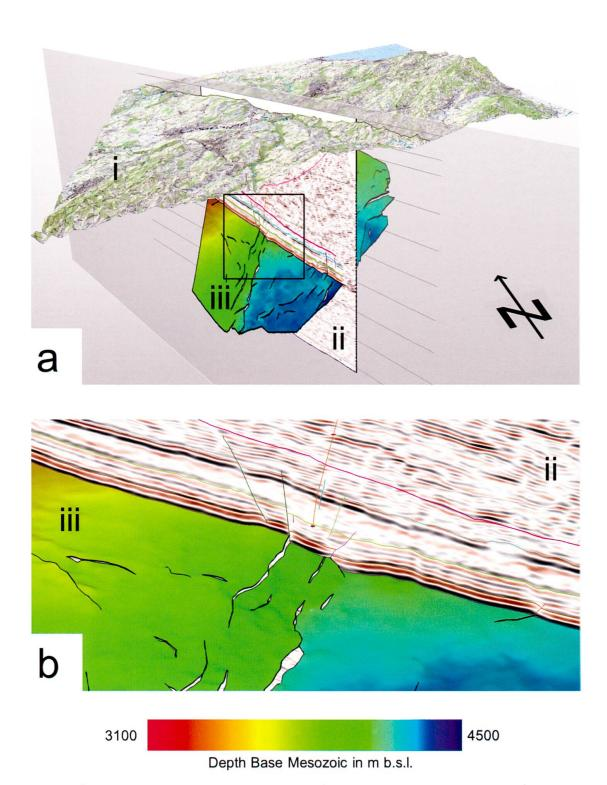
Fig. 4: a] 3D perspective view from South-West (two times vertically exaggerated) of several elements of the 3D model of the St.Gallen area: (i) Topographic map draped onto digital elevation model, (ii) section along SG GT-1 well track (orange subvertical line) showing the depth converted 3D seismic (CRS PSTM stack), and the intersection with all interpreted horizons and faults, (iii) illuminated horizon surface of Base Mesozoic in depth. The black rectangle represents the zoomed area in b].
