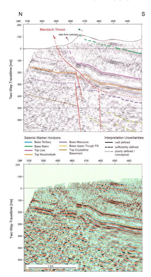
Fig. 5: Mandach Thrust above the northern boundary of the Permo-Carboniferous Trough on seismic section 11-NS-04. For location see Fig. 1.
