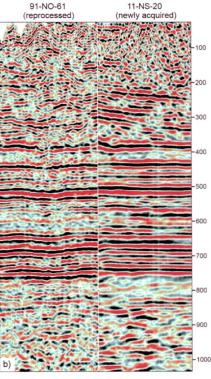
Fig. 2: Comparison of the data quality between reprocessed seismic data of the campaigns 1982/91 and the newly acquired seismic data 2011/12. For location of the sections see Fig. 1.
