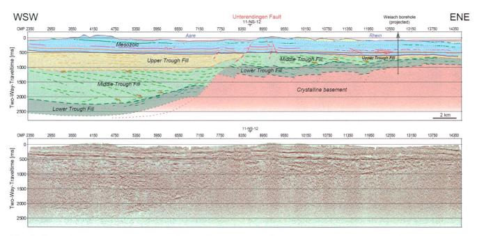
Fig. 4: Key seismic section along the Permo-Carboniferous Trough and interpretation of the Trough fills (adapted from Naef & Madritsch 2014). For location see Fig. 1 and for seismic marker horizons and classification of interpretation uncertainties see Fig. 5.
