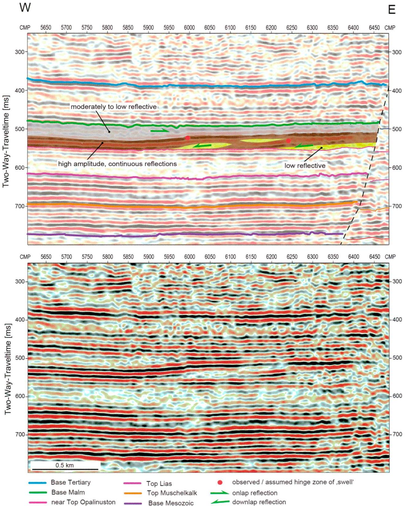
Fig. 7: Reflection geometries and seismic facies changes within the Mid-Upper Dogger sequence outlining a «swell area» in the Nagra siting region «Nördlich Lägern». For location see Fig. 1.
