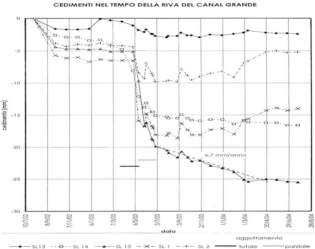
Fig. 8: Time-settlement curves of several anchorages (x-axis: date, y-axis: settlement in mm).
