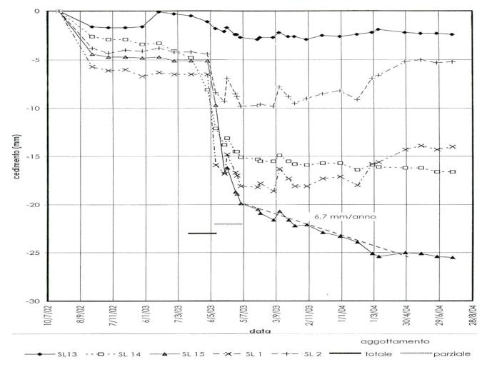
Fig. 8: Time-settlement curves of several anchorages (x-axis: date, y-axis: settlement in mm).
