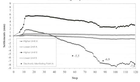
Fig. 6: Time-settlement calculated curves and real measurements at Città di Castello tower.
