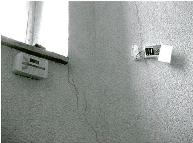
Fig. 15: Easy Crack Monitor System®.
