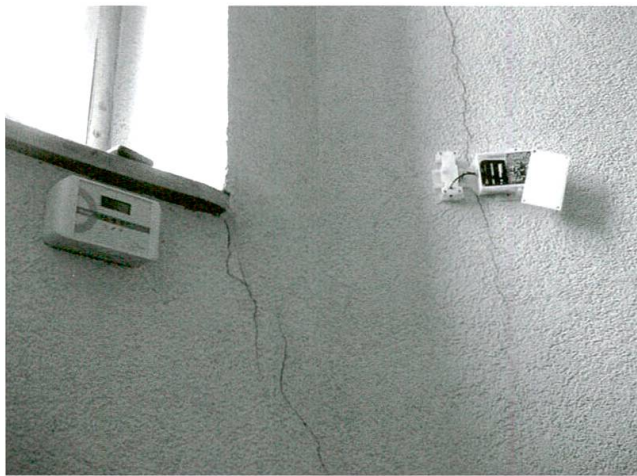
Fig. 15: Easy Crack Monitor System®.
