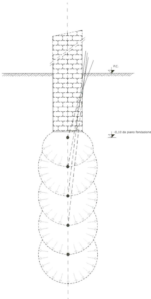
Fig. 3: Injection procedure.
