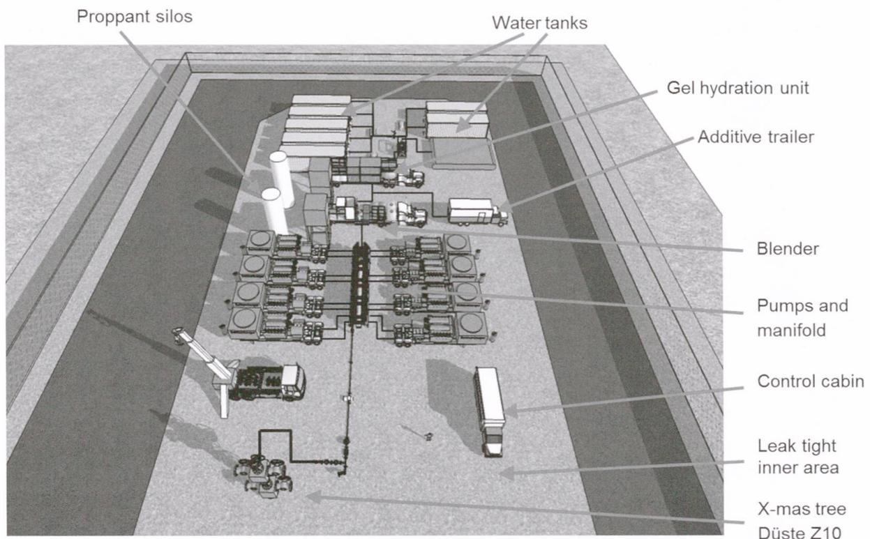
Fig. 6: Layout of fracturing equipment in inner area of Düste Z10 well site.
