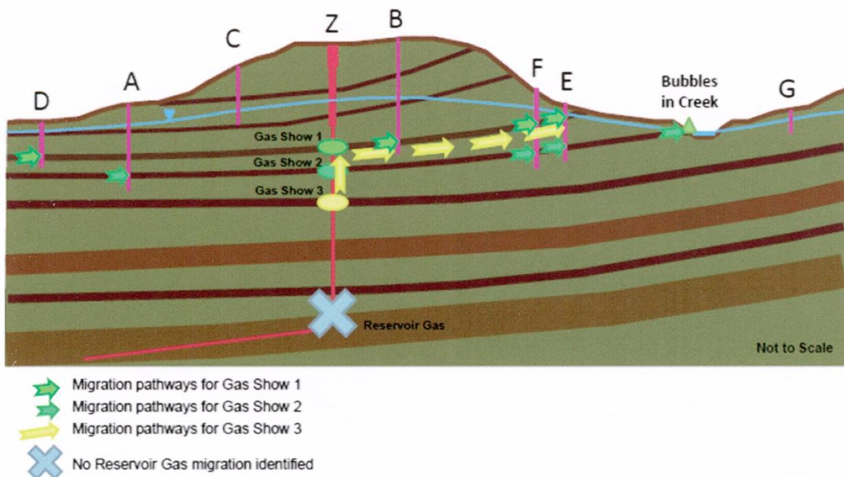
Fig. 3: Stray Gas Forensics to distinguish methane in water well sample from multiple unrelated methane sources (Sueker et al. 2012).
