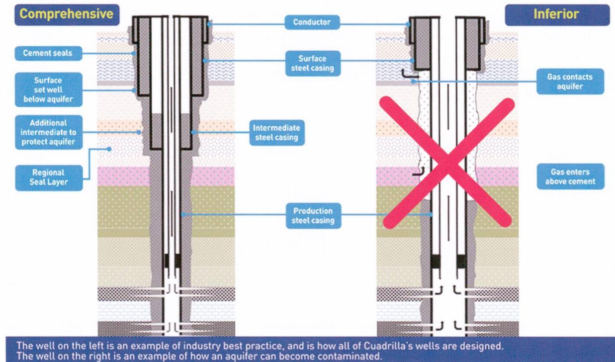
Fig. 8: Well design with and without intermediate casing [Cuadrilla 2014].
