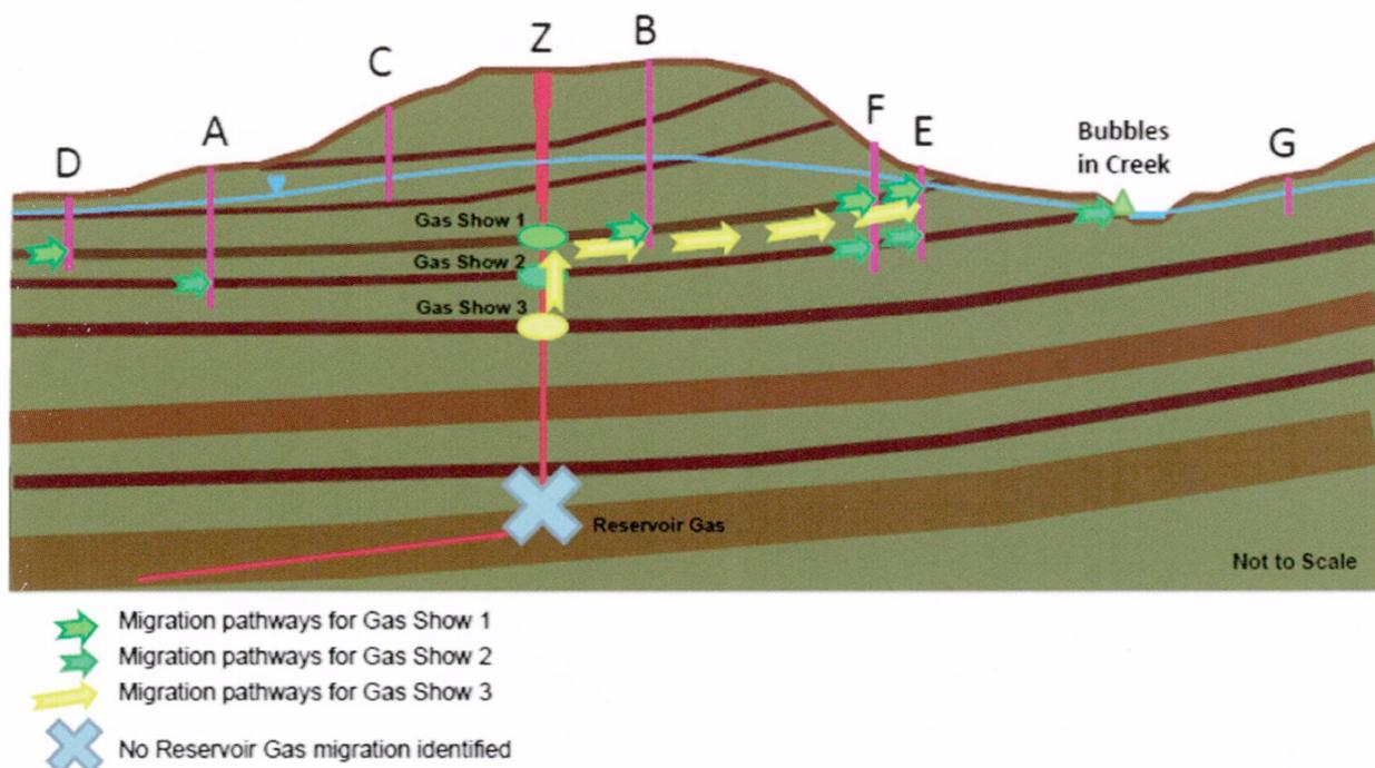
Fig. 3: Stray Gas Forensics to distinguish methane in water well sample from multiple unrelated methane sources including thermogenic sources (Sueker et al. 2012).
