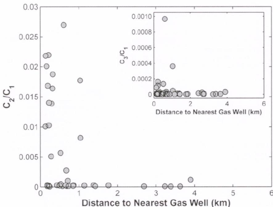
Fig. 5: The ratio of ethane/methane ( $C_2/C_1$ ) and (inset) propane/methane ( $C_3/C_1$ ) concentrations in drinking water wells as a function of distance to natural gas wells (kilometers) (Jackson et al. 2013).
