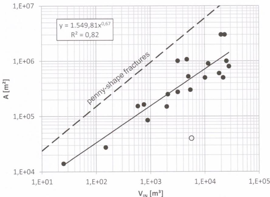
Fig. 9: Area of the seismic clouds of all major EGS-projects vs. injected volume (after Jung 2013). Fitting line and coefficient of determination  $R^2$  is for the solid data points. Open circle: Data point of a gel-frac test in well RH-15 of the Camborne system. Dashed line: Trend-Line for penny-shape fractures for  $E' = 50$  GPa and  $K_{IC} = 1.5$  MPa·m<sup>1/2</sup>.
