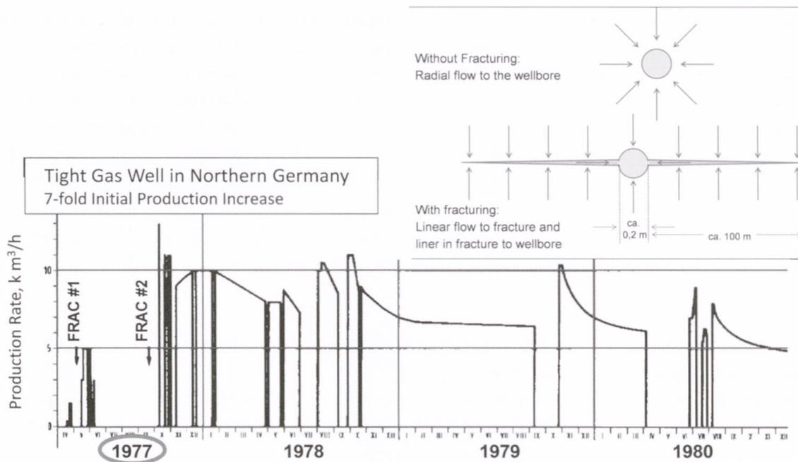
Fig. 4: Effect of a hydraulic fracturing treatment on flow pattern and well productivity (in 1.000 m<sup>3</sup>/h).
