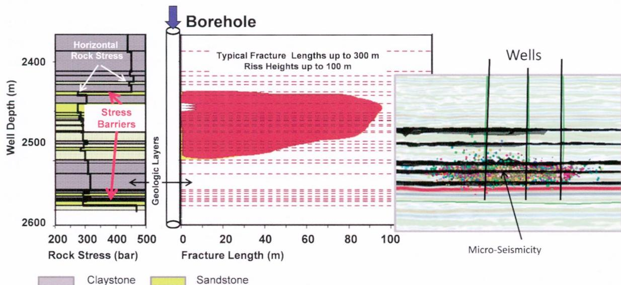
Fig. 1: Fracture propagation in a reservoir: left prognosis, right measurement. The prognosis of fracture propagation is made with recognized methods and commercially available simulators based on the knowledge of the geo- and hydro-mechanical properties of the subsurface and its stress distribution. The measurement is made by monitoring the micro-seismicity associated with the fracture extension [right].
