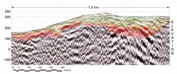
Hybrid seismic section by overlaying the refraction tomography velocity field onto the reflection seismic depth section
