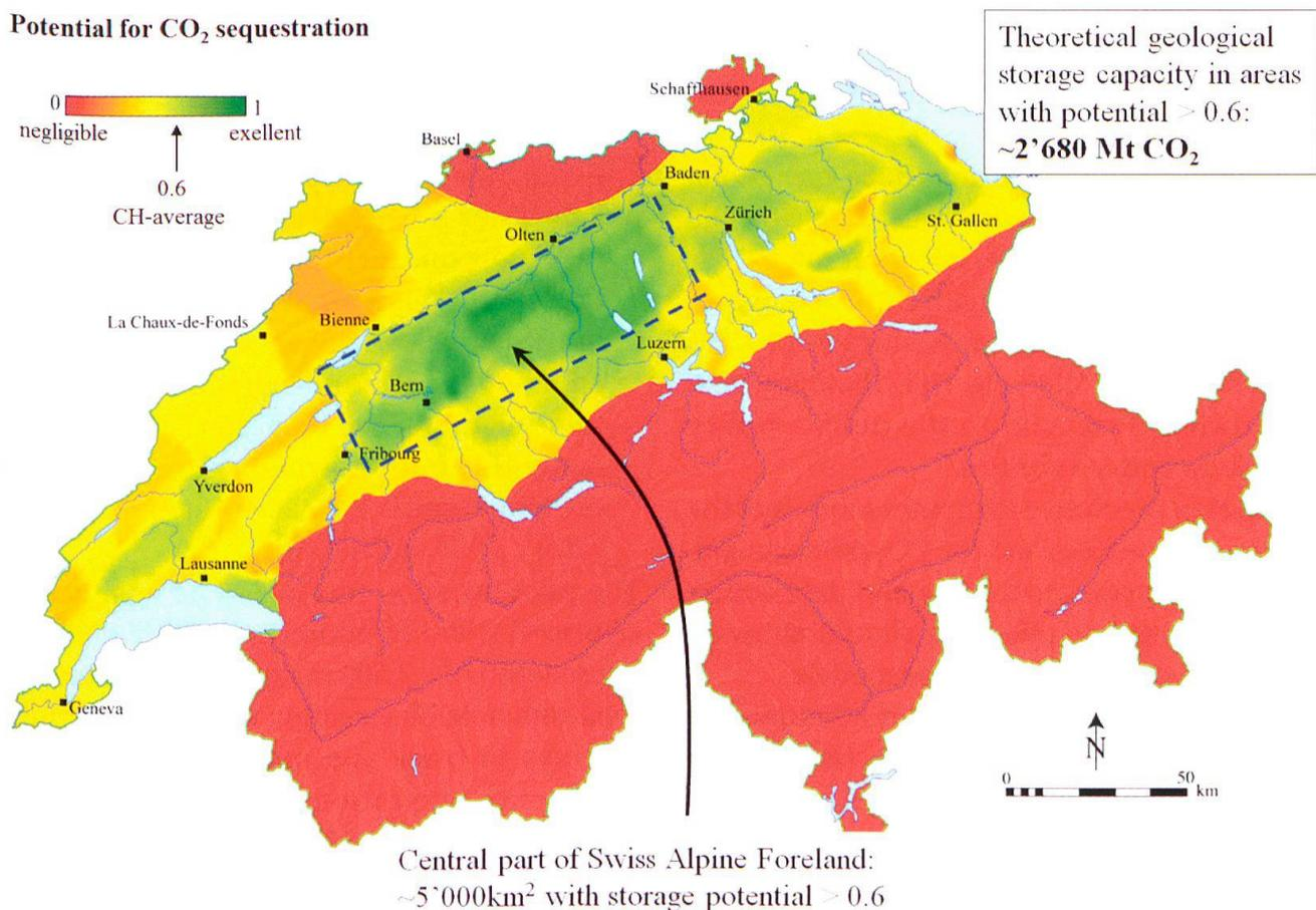
Fig. 2: Technical geological potential for CO<sub>2</sub> sequestration in deep saline aquifers of Switzerland. The combined storage capacity of the four main aquifers with a potential of > 0.6 amounts to a total of ~ 2,670 million tons of CO<sub>2</sub> and is concentrated mainly in the central part of the Alpine Foreland south of the Jura (modified from Diamond et al. 2010).
