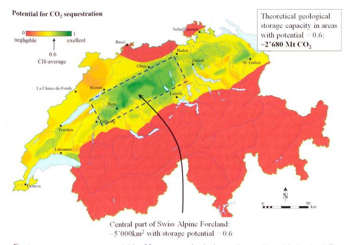
Fig. 2: Technical geological potential for  $CO_2$  sequestration in deep saline aquifers of Switzerland. The combined storage capacity of the four main aquifers with a potential of > 0.6 amounts to a total of ~ 2,670 million tons of  $CO_2$  and is concentrated mainly in the central part of the Alpine Foreland south of the Jura (modified from Diamond et al. 2010).
