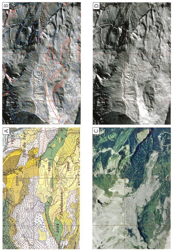
Fig. 5: Comparison between an ancient map sheet of the GA25 with swissALTI<sup>3D</sup> and ortho image. [A] ancient geological map (extract of map 35 St-Léonard; Badoux et al. 1959); [B] geological contours of the vectorized map and underlying swissALTI<sup>3D</sup>; [C] ortho image; [D] hillshade view based on swissALTI<sup>3D</sup>.
