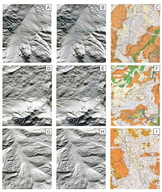
Fig. 4: Analysis and interpretation of quaternary landforms using hillshade view based on swissALTI<sup>3D</sup> and presentation on a geological map (extract of map 122 Vissoie; Marthaler et al. 2008). [A] – [C] gravitational and fluviatile deposits; [D] – [F] glacial and periglacial deposits; [G] – [I] slope instabilities. See text for legend.
