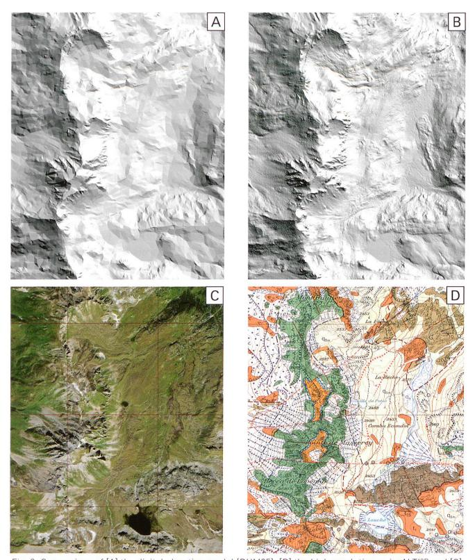
Fig. 3: Comparison of [A] the digital elevation model (DHM25); [B] the high resolution swissALTI<sup>3D</sup> and [C] ortho image used for interpretation and mapping of quaternary landforms displayed on a [D] geological map (extract of map 122 Vissoie; Marthaler et al. 2008).
