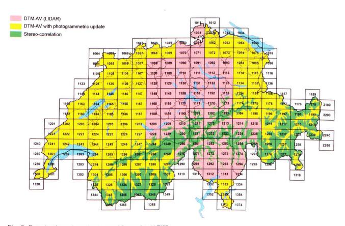
Fig. 2: Data basis and methods used for swissALTI3D.
