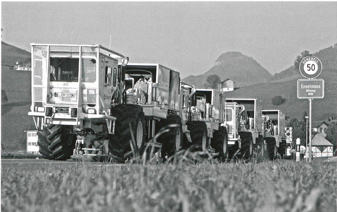
Fig. 2: Convoy of vibrotrucks recording in Nidwalden.
