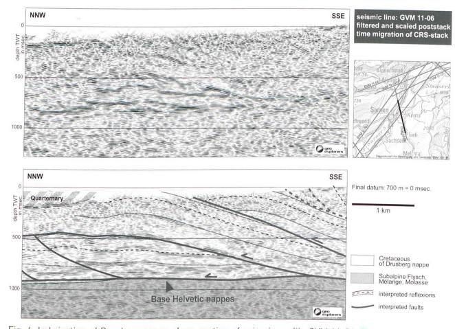
Fig. 6: Imbrication of Drusberg nappe along section of seismic profile GVM 11-06. The cross section is inclined to structural strike of folding and thrusting. Therefore dip of thrusts appears gentle and displacement is exaggerated. Interpretation on the upper right hand part of profile is based on surface geology.
