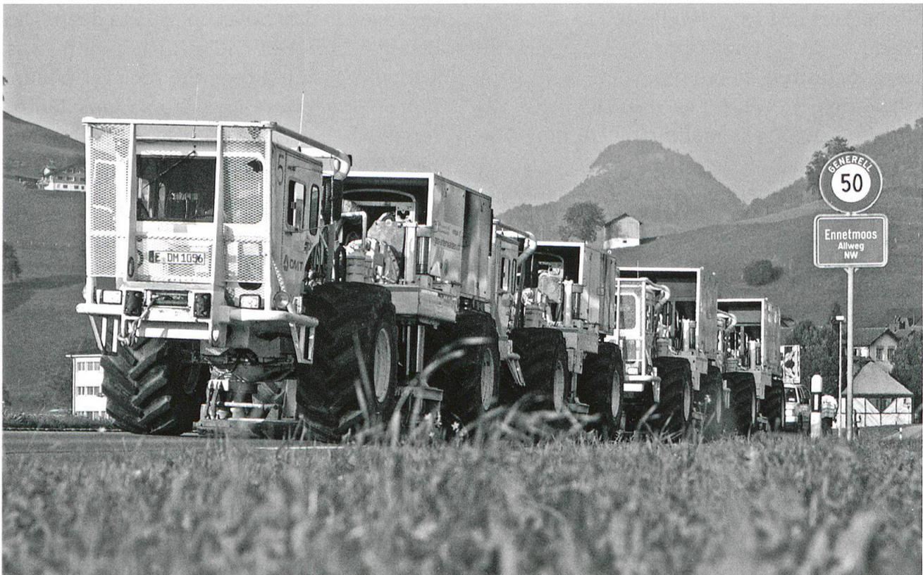
Fig. 2: Convoy of vibrotrucks recording in Nidwalden.
