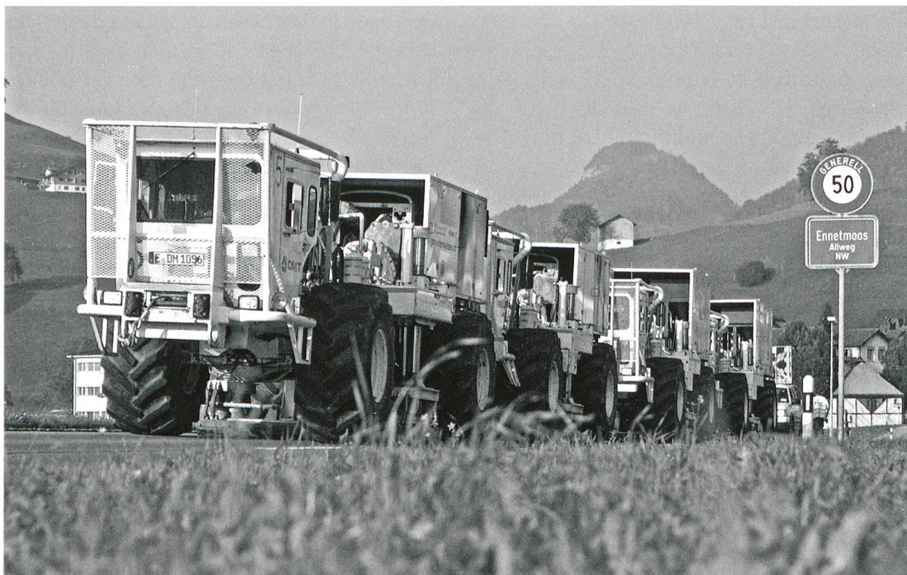
Fig. 2: Convoy of vibrotrucks recording in Nidwalden.
