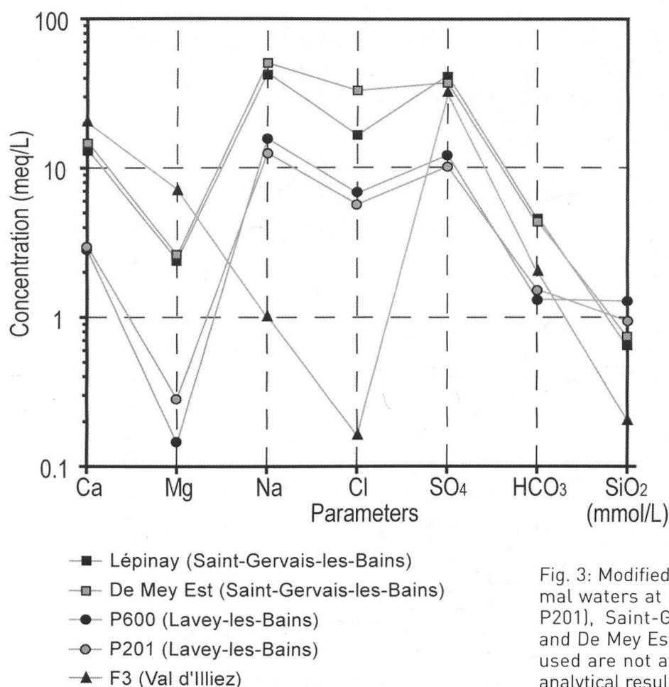
Fig. 3: Modified Schoeller diagram of thermal waters at Lavey-les-Bains (P600 and P201), Saint-Gervais-les-Bains (Lépinay and De Mey Est) and Val d'Illicz (F3). Data used are not average values but discrete analytical results found in Sonney (2010).
