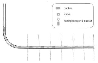
Fig. 9: Hydraulic fracturing. Scheme of a multipacker assembly for shale gas wells. The valves can be activated individually so that one fracture after the other can be created starting from the bottom of the well.
