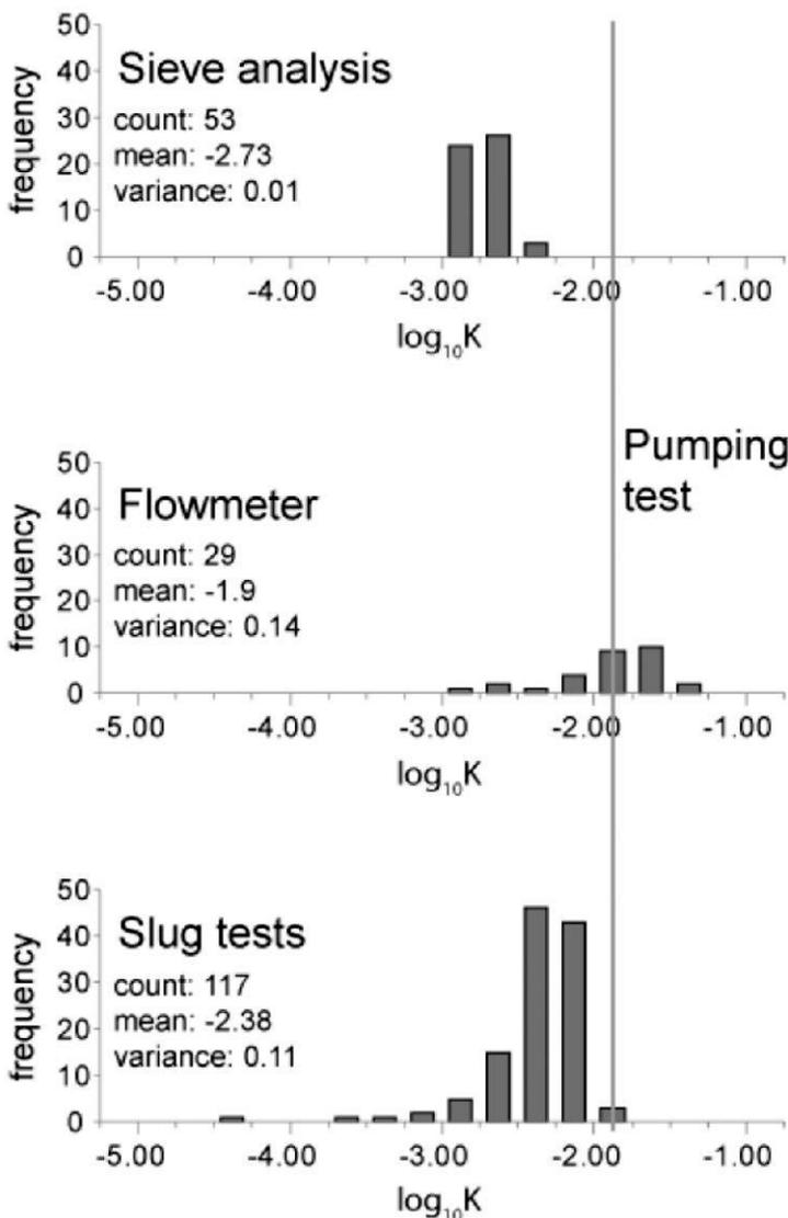
**Fig. 2:** Histograms of logarithmic hydraulic conductivity with indicated number of datapoints [count], logarithmic geometric mean and logarithmic variance (modified after Diem et al. 2010).
