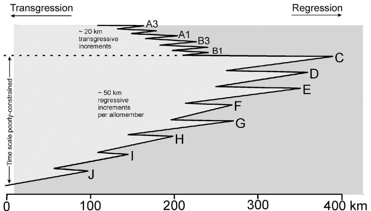
**Fig. 5:** Summary of generalized shoreline movements during deposition of the Dunvegan Formation, based on detailed paleogeographic maps in Plint 2000. Vertical time-scale is poorly-constrained; it seems likely that the entire formation was deposited in less than about two million years. Unpublished data suggest that the sequences in allomembers A and B may have been of shorter duration than those shown for allomembers J to C [based on Plint 2000 and Hay & Plint 2009].
