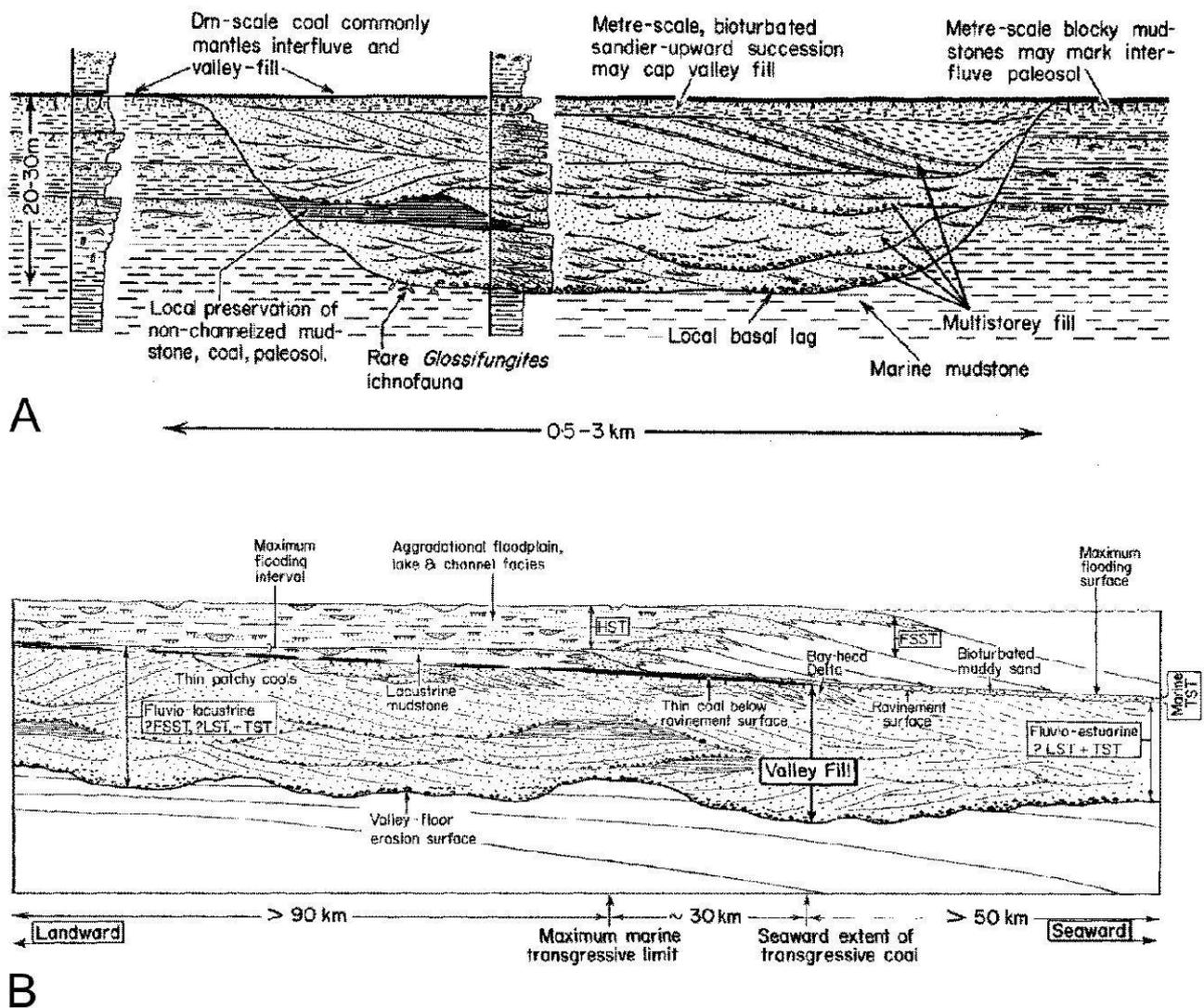
**Fig. 4:** A) Principal characteristics of Dunvegan paleovalley-fills seen in transverse view [from Plint & Wadsworth 2003]. B) Principal characteristics of Dunvegan paleovalley-fills seen in longitudinal view [from Plint & Wadsworth 2003]. The strata are divided into transgressive, highstand, falling stage and lowstand systems tracts.
