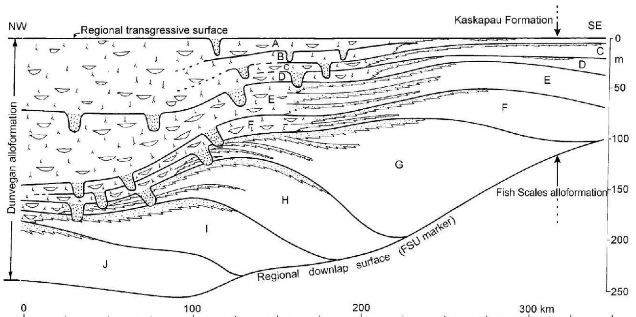
**Fig. 3:** Summary stratigraphic diagram, drawn to scale, showing the geometry and broad facies distribution of Dunvegan allomembers J-A in a NW-SE dip-oriented section (from Plint & Wadsworth 2003). Paleovalleys are incised into the top surfaces of most allomembers [which can also be interpreted as depositional sequences].
