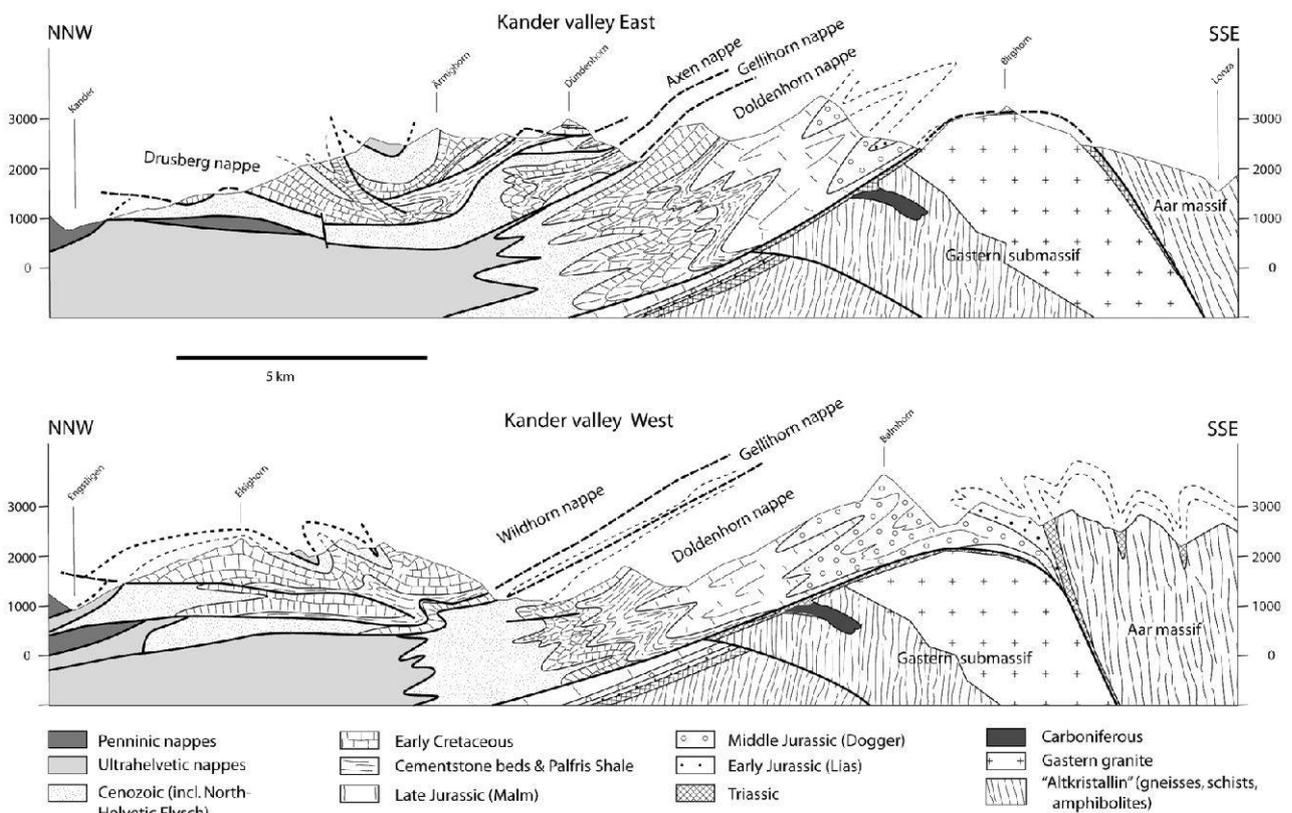
**Fig. 2:** Geological profiles across the Helvetic nappe system east and west of the Kander valley. Traces are given in Fig. 1. Whereas the Doldenhorn nappe and the underlying basement uplifts show a similar structure, the Doldenhorn nappe is much more voluminous on the eastern side and the structures within the Axen-Drusberg and the Wildhorn nappes are entirely different.
