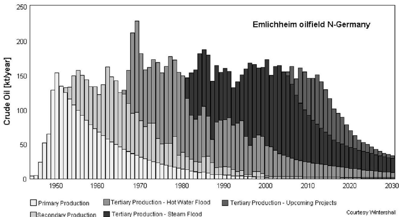
**Fig. 4:** Impact of enhanced oil recovery. Emlichheim heavy oil field North Germany. Thanks to continuously improving technology Emlichheim has been producing at economic rates for over 60 years, increasing the recovery rate from 7% to 33% [courtesy Wintershall AG].
