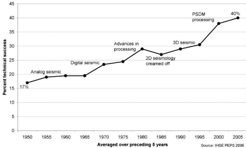
**Fig. 2:** Exploration wildcat technical success rates 1946 - 2005 and impact of developments in seismic technology (adapted from K. Chew, IHS).
