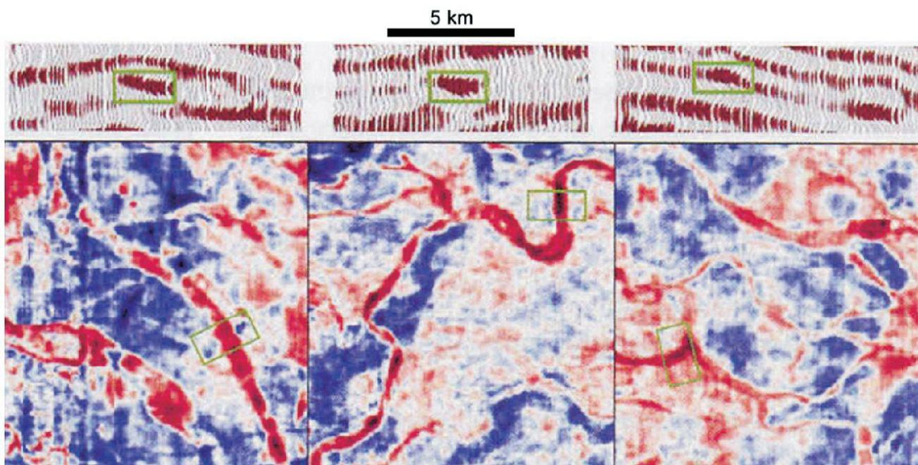
**Fig. 8:** Progress in seismic imaging: reservoir identification. Special processing and attribute displays enhance subtle features like the river channels, shown only as small anomalies in the sections at the top [Chopra & Marfurt 2007].
