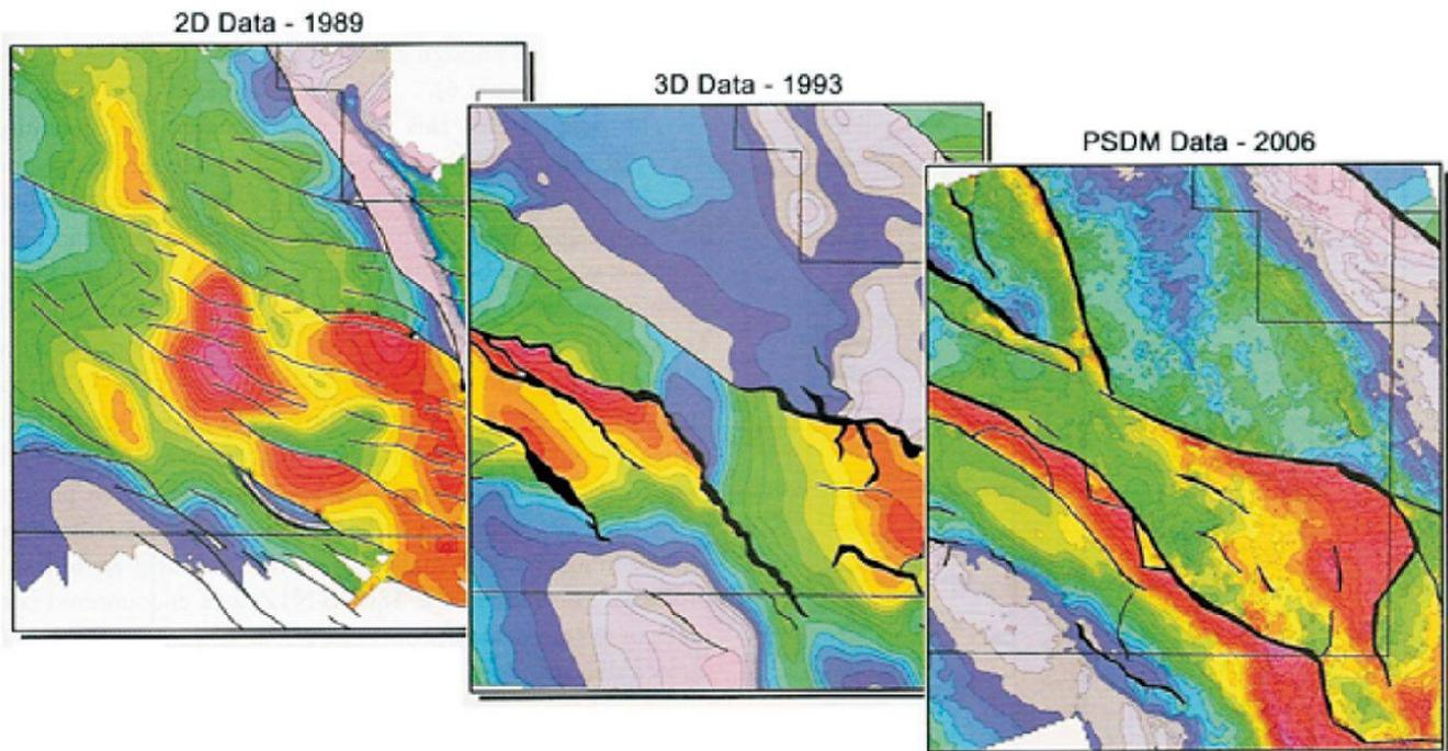
**Fig. 10:** Progress in seismic imaging: structural definition. Different interpretations of a North Sea field, based on 2D seismic, 3D seismic and Prestack Depth Migration (PSDM). Note dramatic difference/improvement introduced by PSDM, showing that 2D and conventional processing of 3D was not able to resolve a complex tectonic pattern (Elam 2007).
