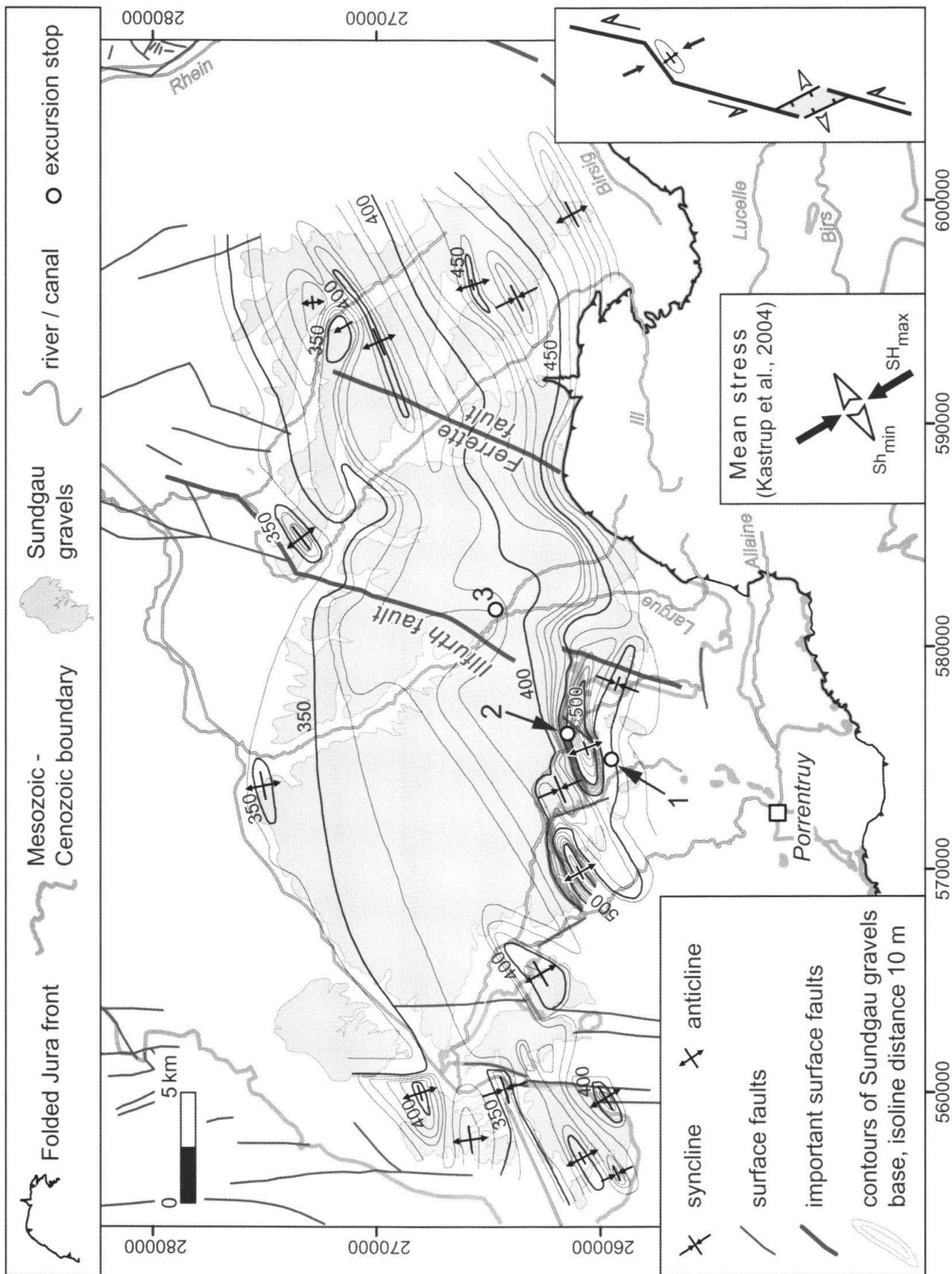
**Fig. 2:** Contour map of the base of the Pliocene Sundgau gravels in metres above sea level (after Giamboni et al. 2004a). Bottom right inset: kinematic sketch of the Illfurth fault explaining the occurrence of restraining and releasing bends. VSP-ASP convention 2006 excursion stops are indicated.
