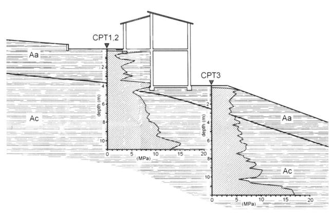
Fig. 6: Soil profile and CPT initial results.
