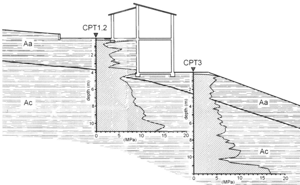
Fig. 6: Soil profile and CPT initial results.
