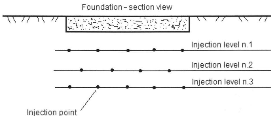
**Fig. 3:** Schematic representation of the Urettek injection procedure.
