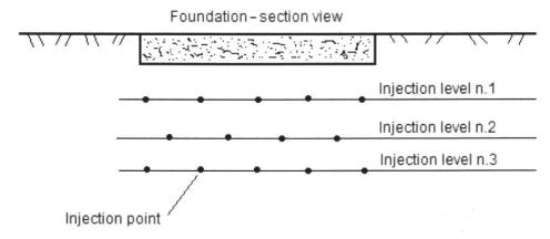
Fig. 3: Schematic representation of the Uretek injection procedure.
