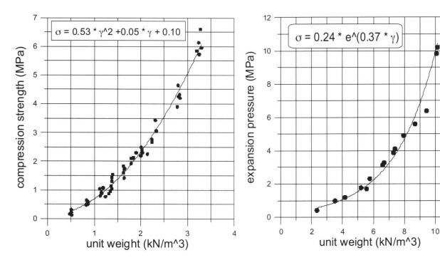
Fig. 1: Uniaxial compression test results: vertical stress  $\sigma$  vs. sample unit weight  $\gamma$ .
