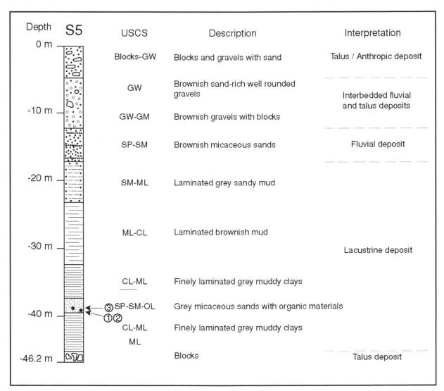
**Fig. 3:** Simplified stratigraphic log of the Cavienca S5 borehole with emplacement of the dated samples.
