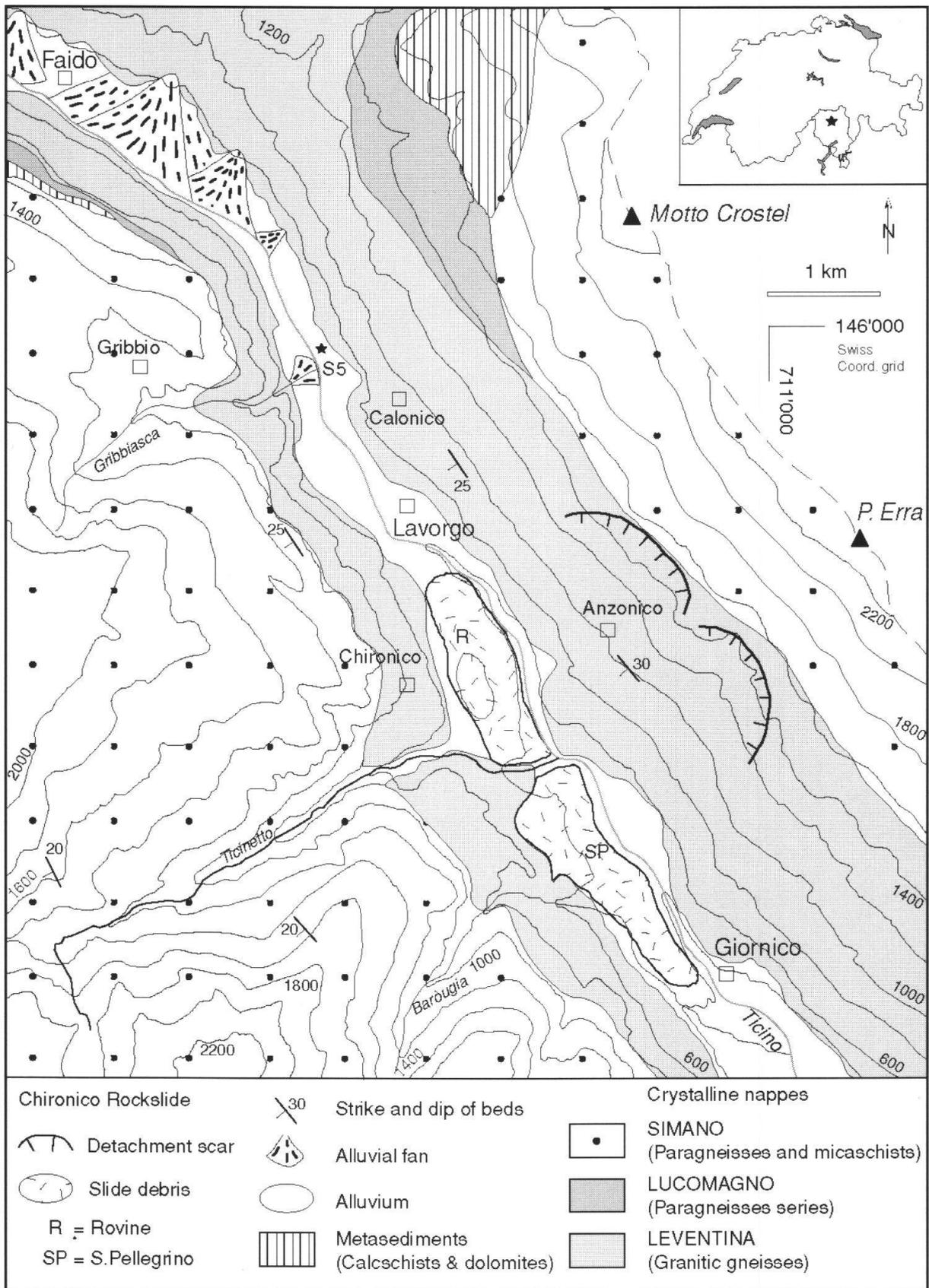
**Fig. 1:** Tectonic sketch map of central Leventina with location of the Chironico rockslide. Dashed line is the eastern side of the watershed. \*S5 shows drilling location. Compiled after Nägeli (1920), Bianconi (1971) and Keller et al. (1980).
