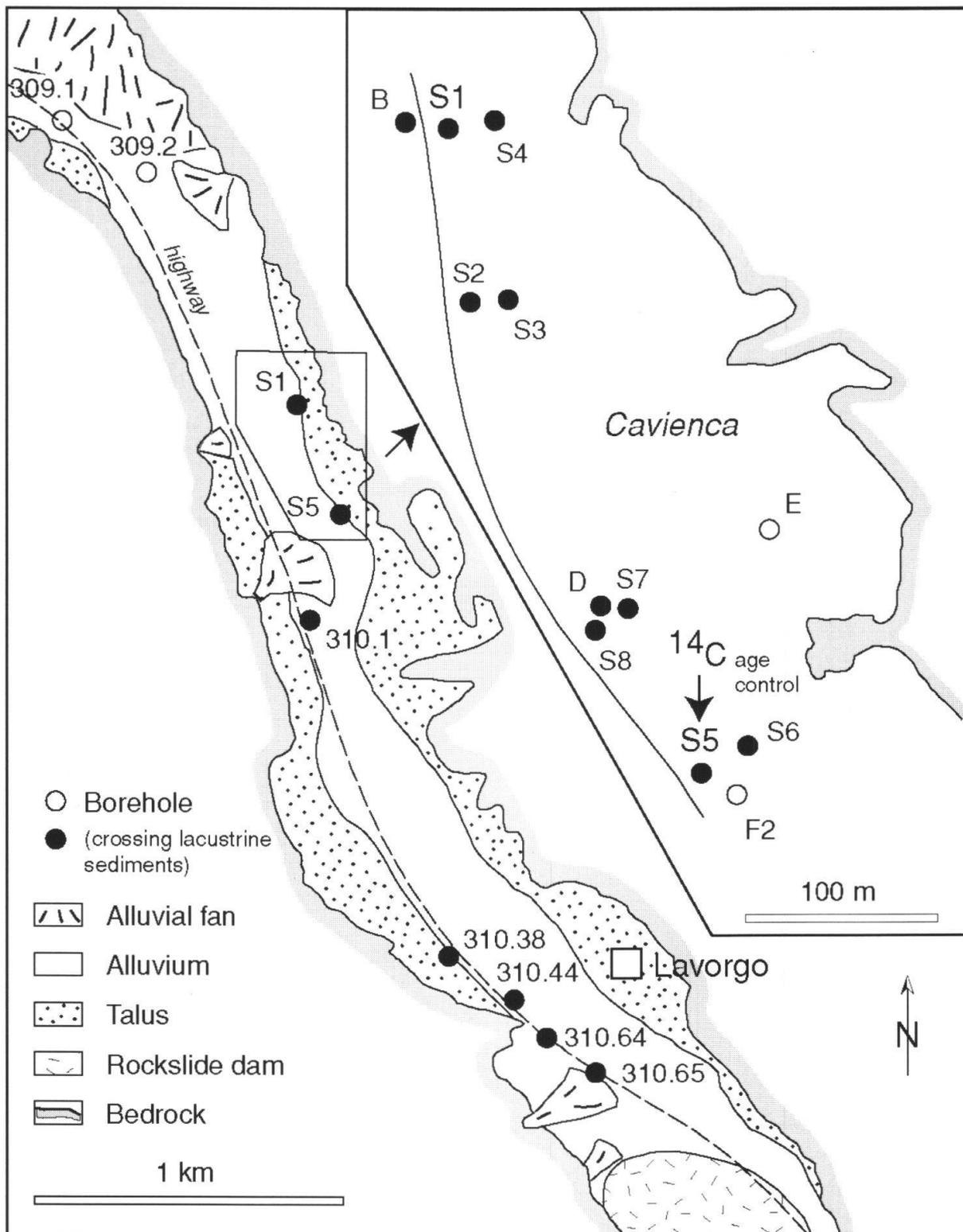
**Fig. 2:** Map showing the general layout of the drillings carried out in the alluvial plain to the north of Lavorgo. Inset shows a simplified general site map of Caviencia landfill with location of the drillings of 1997 and 2001.
