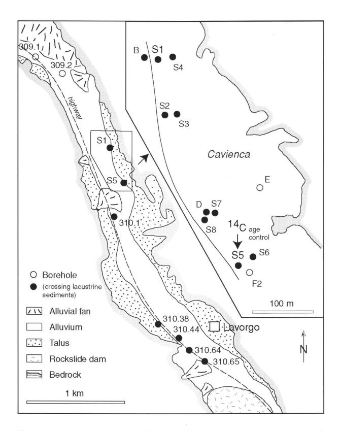
**Fig. 2:** Map showing the general layout of the drillings carried out in the alluvial plain to the north of Lavorgo. Inset shows a simplified general site map of Cavienca landfill with location of the drillings of 1997 and 2001.
