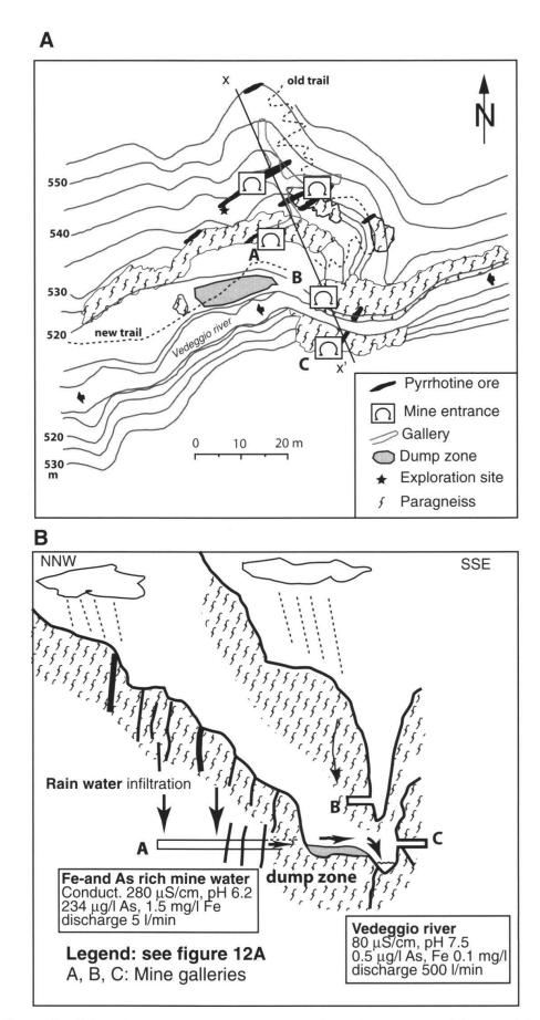
Fig. 11: Example of the release of arsenic by mine galleries and dump material: case of the pyrrhotine mine W of Medeglia (geology updated after Fehlmann 1919 and Kündig et al. 1990).
