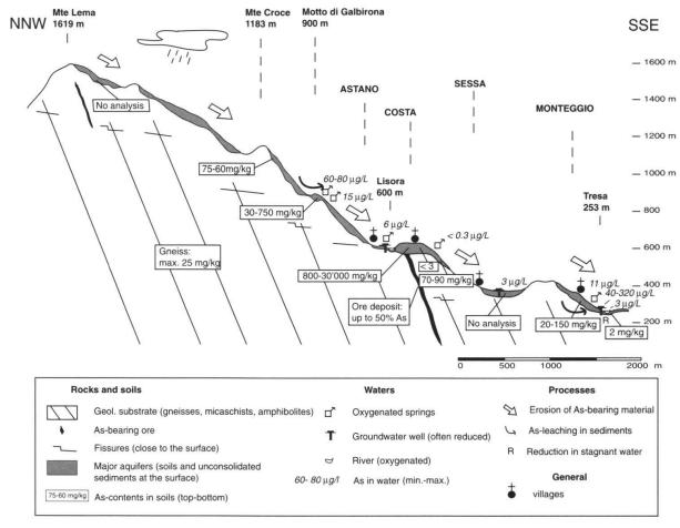
**Fig. 8:** Cross-section of the Malcantone area, schematically summing up the different situations in which arsenic has been found in rocks and waters: waters rich in As are not directly linked to ore deposits. On slopes oxygenated waters with medium contents dominate, whereas in locally reduced ground waters related to river plains high As-values can be found.
