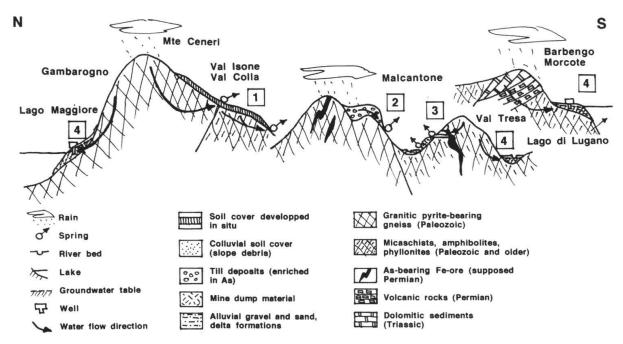
**Fig. 3:** Very schematic geological cross section through the Sottceneri region, showing the different hydro-geological situations in which the waters with elevated arsenic contents occur. The four general aquifer situations indicated (with numbers 1 to 4) are explained in detail in figure 4.
