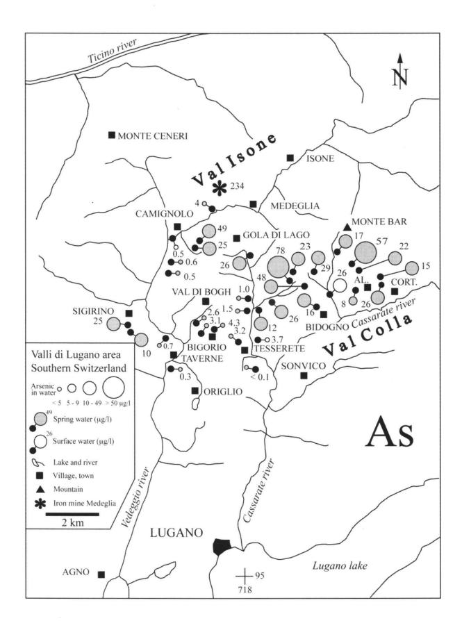
Fig. 9: Arsenic contents in waters of the Valli di Lugano area (Val Isone-Val Colla). The concentrations are comparable to the Malcantone area, however, Fe-ore deposits which could be at the origin of the elevated arsenic contents are almost absent (only case: pyrrhotine mine of Medeglia). Abbreviations: Cort. Corticiasca, Al.: Albumo.
