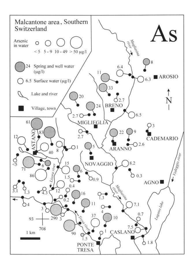
Fig. 7: Arsenic contents in spring, surface and river plain ground waters in the Malcantone area. The size of the circles is proportional to the concentration in  $\mu$ g/l. Towards the east and the south the concentrations are clearly diminishing.
