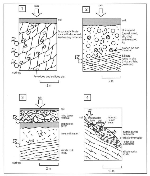
Fig. 4: The four main types of aquifers producing waters with elevated arsenic contents.
