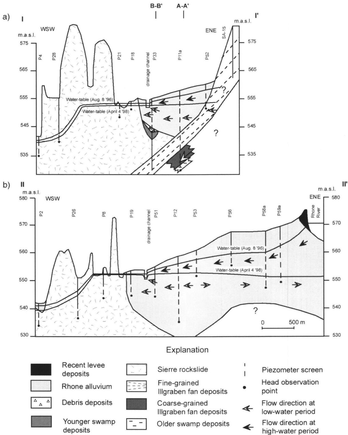
**Fig. 2:** Geologic cross sections a) I-I' and b) II-II' along the Rhone River valley and along the principal groundwater flow path. Line of section and borehole locations are shown in Figure 1.
