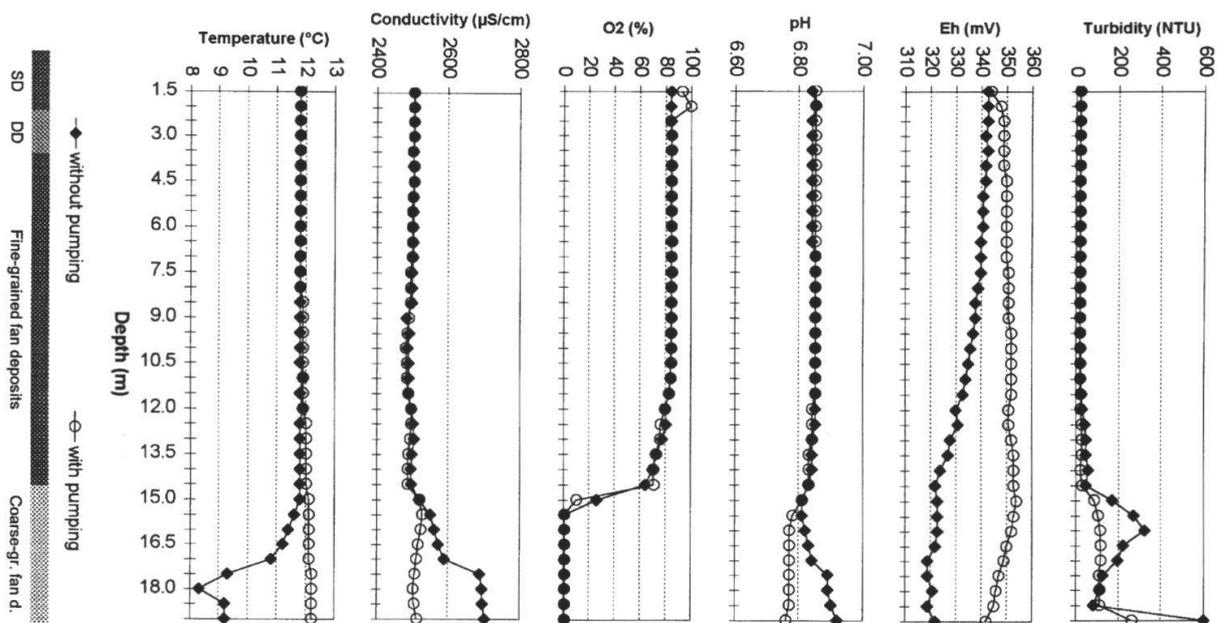
**Fig. 11:** Multiparameter logging in borehole SA-12 on July 15, 1997 under natural conditions (no pumping) and under pumping at about 86.4  $\text{m}^3\text{d}^{-1}$ . SD = Swamp Deposits; DD = Debris Deposits.
