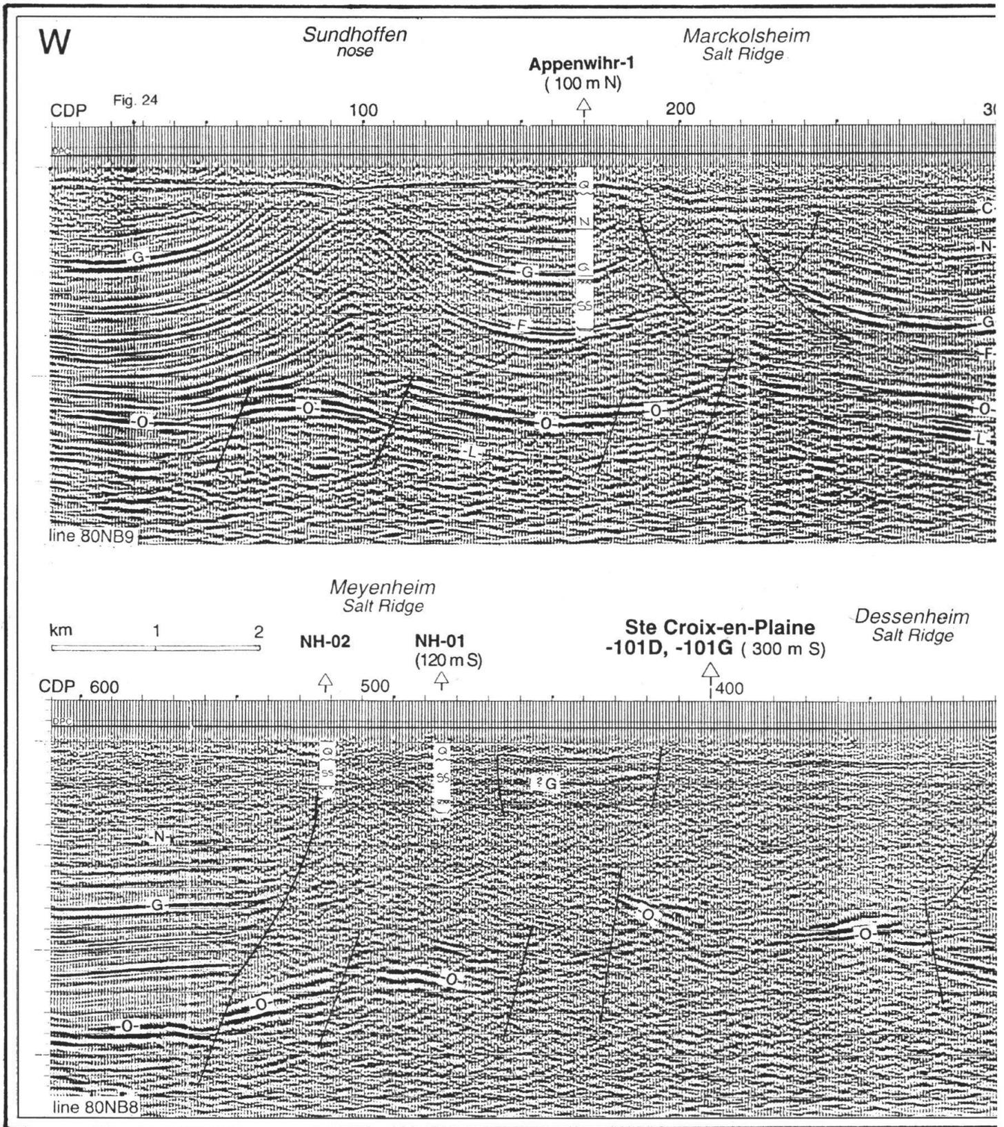
**Fig. 22:** a) Seismic W-E section Sundhoffen - N of Neuf-Brisach;
