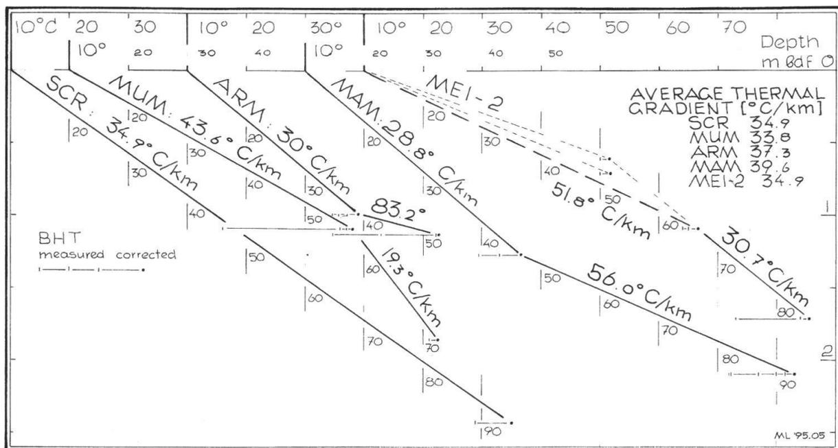
**Fig. 37:** Temperatures and temperature gradients in the wells drilled.
