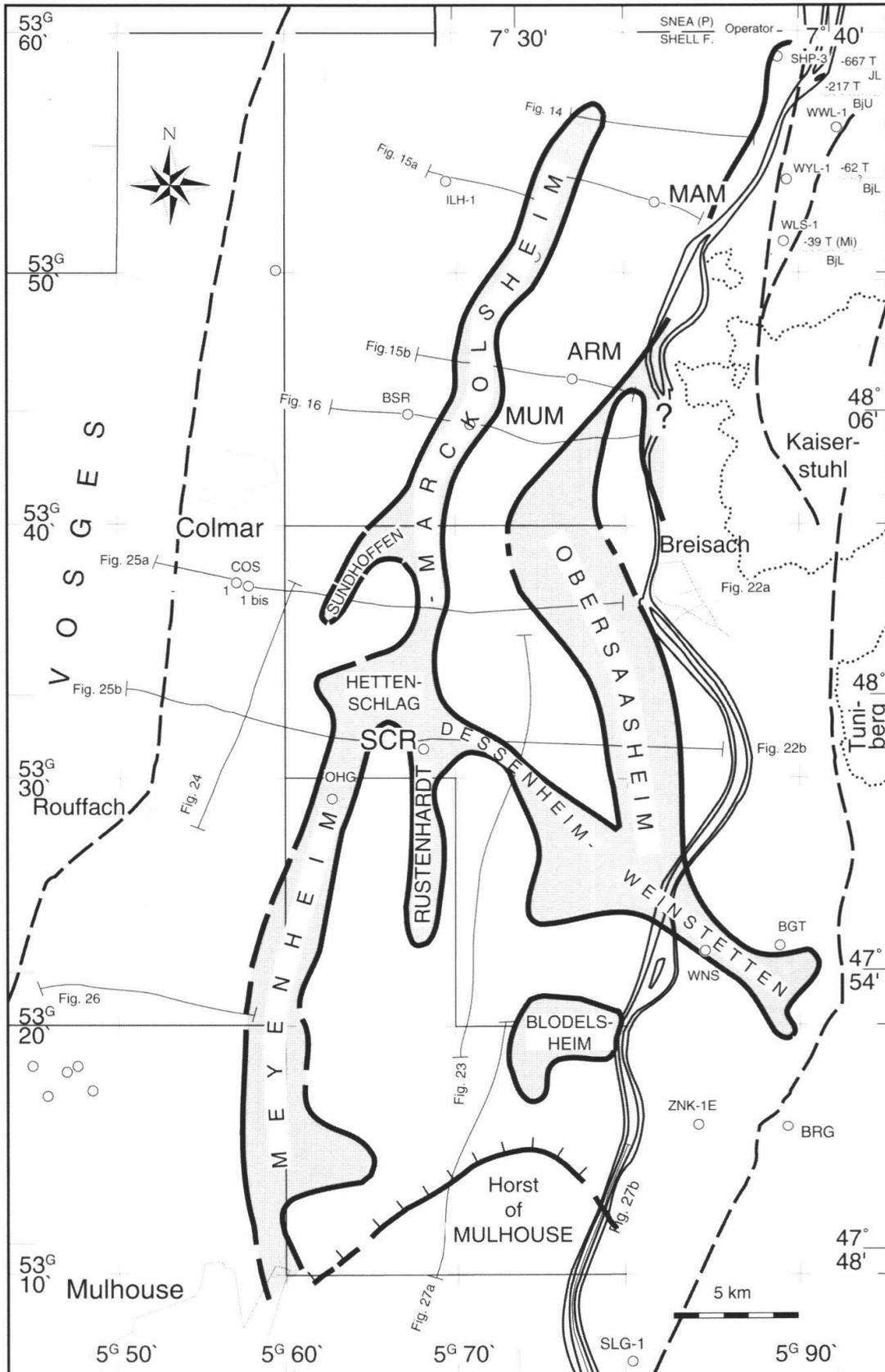
**Fig. 21:** Colmar - Mulhouse area: Subcrop of the Tertiary salt ridges and domes below the Plio- Pleistocene unconformity
