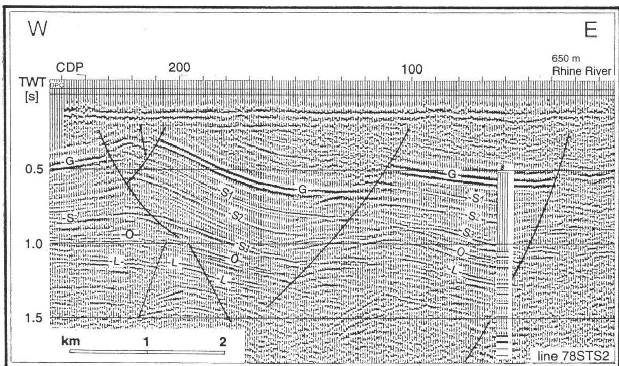
**Fig. 14:** Seismic W-E section N of Mackenheim, just S of a line connecting Artolsheim (F) and Weisweil (D); below CDP 60, synthetic seismogram of the Mesozoic of well MEI-2 used for reflexion identification; location of section on Fig. 12.
