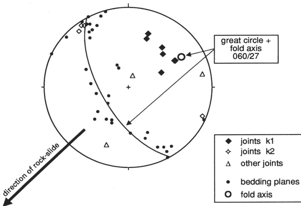
**Fig. 8:** Stereographic projection (lower hemisphere) of joints and bedding planes in the stable area above and behind the rock slide if Nünalpstock-Sörenberg (data be Geotest and von Moos).
