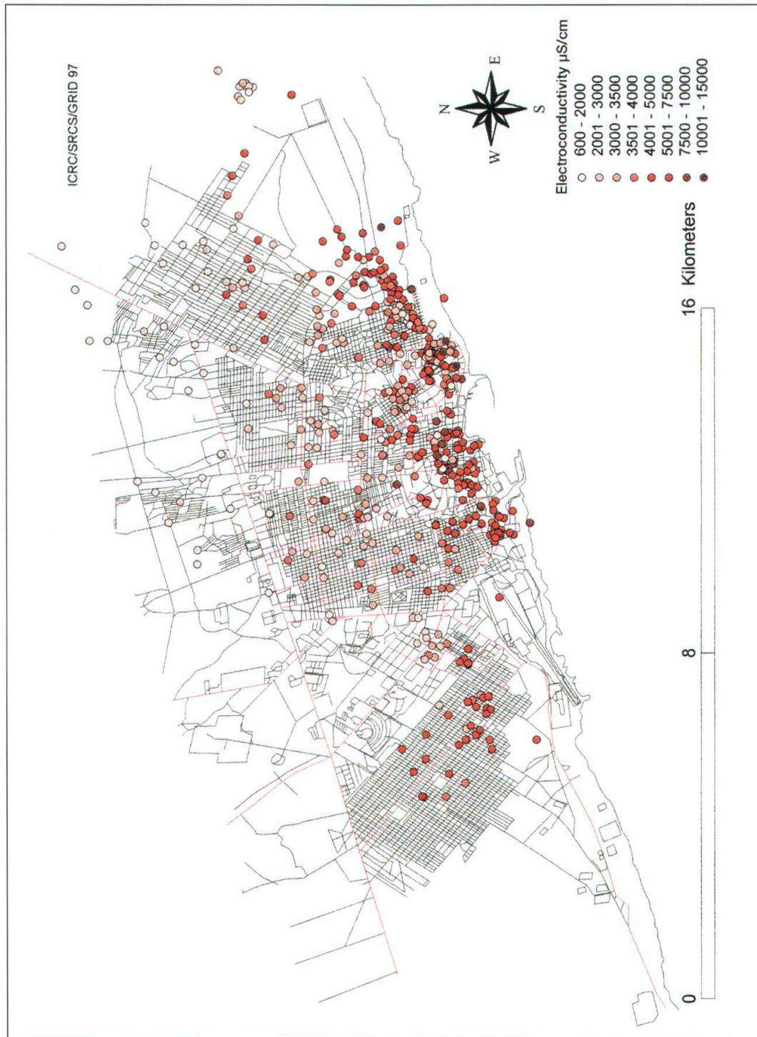
**Fig-4:** Mogadishu: conductivity of groundwater in wells expressed in microS/cm.
